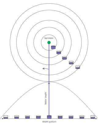
Fig. 3-1- Application pattern of a sprinkler irrigation lines once.
