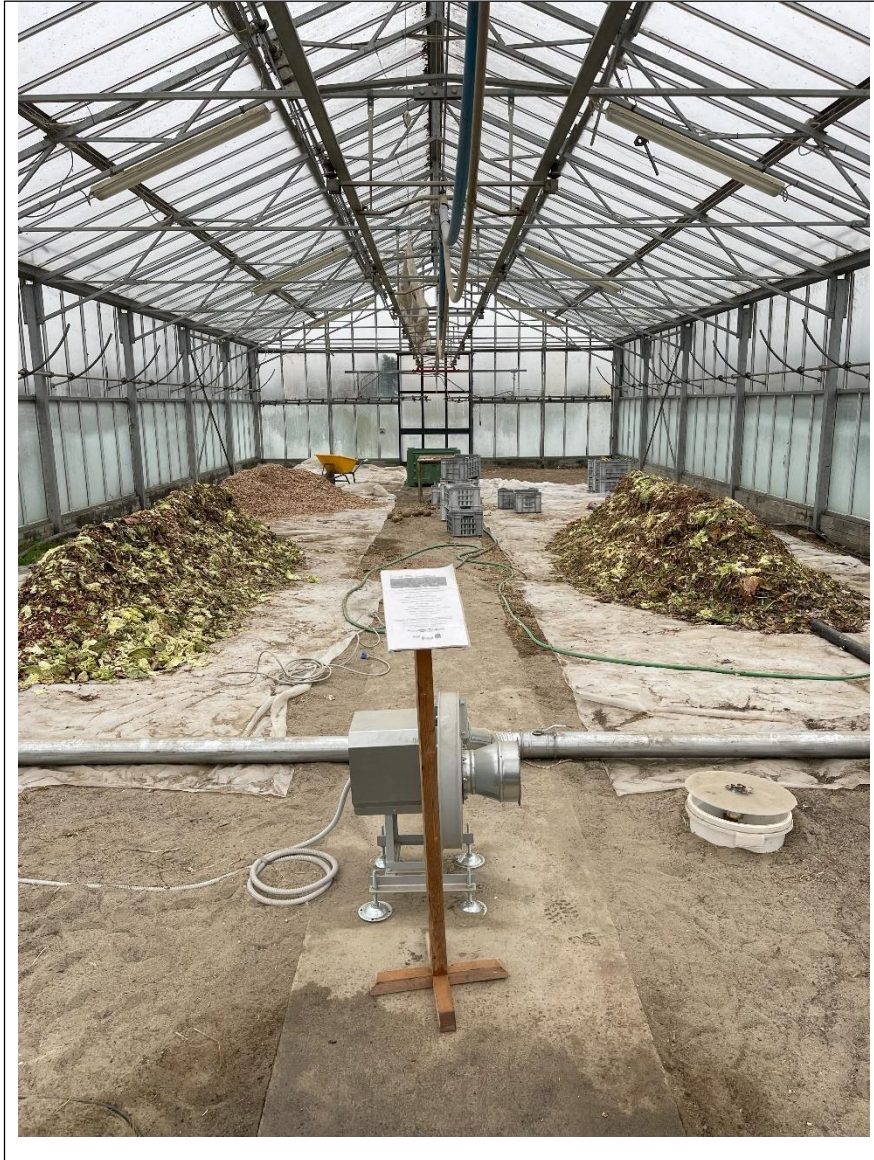
Fig. 2: small-sized pilot plant for compost production (passively aerated static pile)
