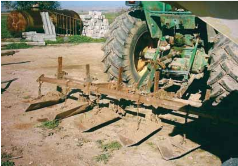
Figure 4.5. Furrowers used on the irrigation strips of the experimental fields.
