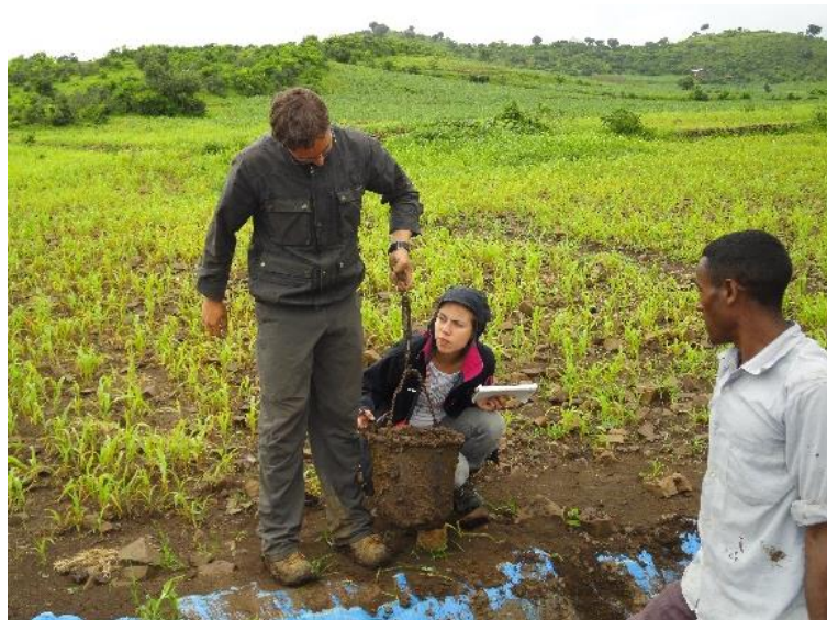
Figure 15: Weighing of the removed sediment using a spring balance
