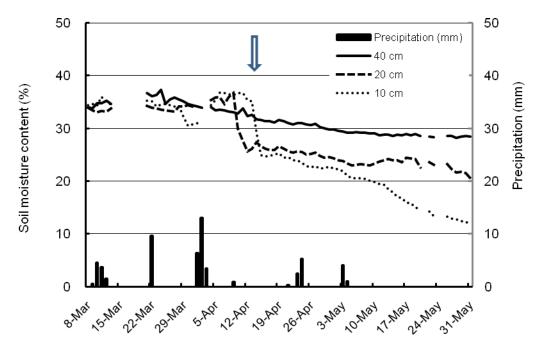
Fig. 3 Soil water content at depths 10, 20 and 40 cm in a field plot of bread wheat genotype "Cham 6", collected through a Field Sever. Arrow indicates the heading time of wheat material.
