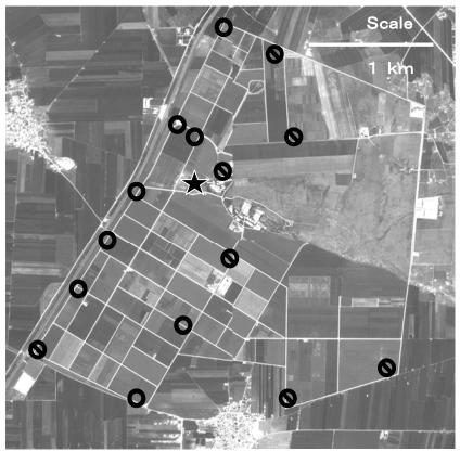
Fig. 2 ICARDA field map showing the distance of wireless transmission between the access point and the Field Server. Access point was located at , and the Field Servers were at (successfully transmitted), or (not transmitted).
