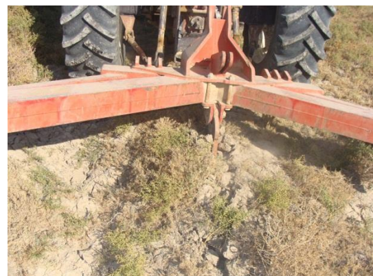
Figure 15. Use of rotor to breakdown hardpan in deep plowing at Dujaila Site.
