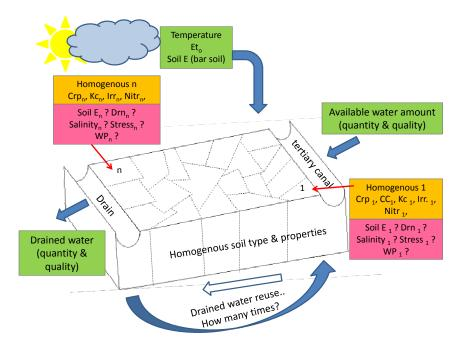
Figure (1): Simplification schematic model of the tertiary canal zone system, where: Crp = crop type, Kc = crop coefficient, Irr = irrigation application, Nitr = nutrition application, Soil E = soil evaporation, Drn = drained water amount, and WP = water productivity.
