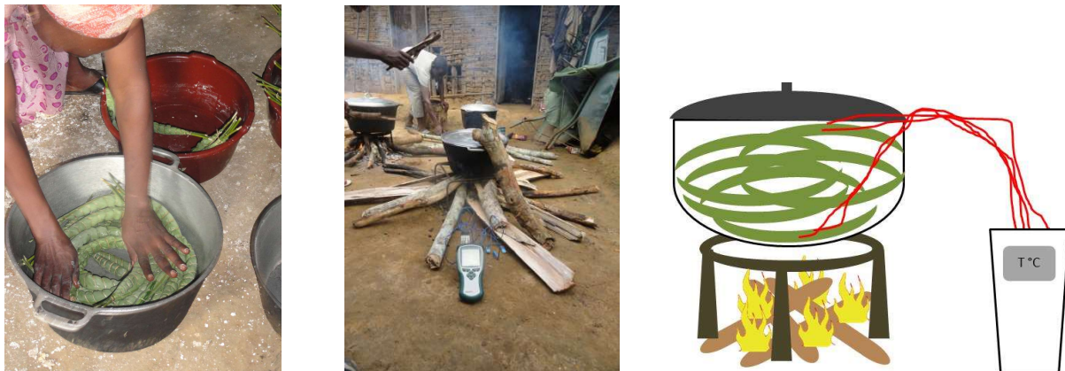
Figure 20: Cooking system instrumentation
