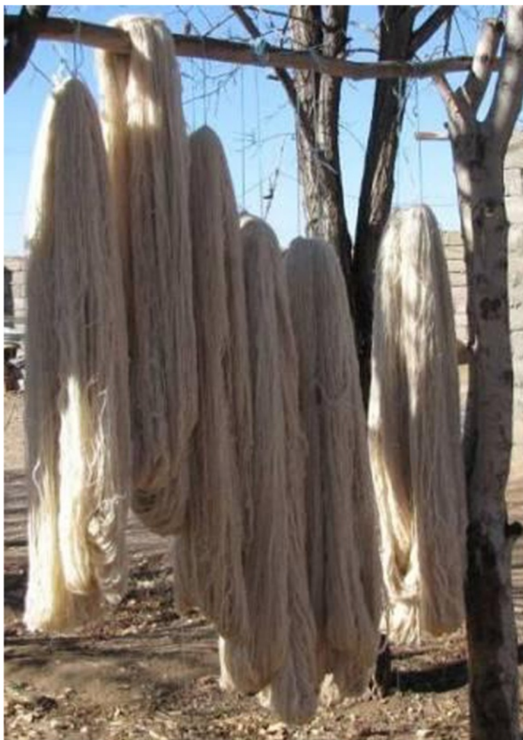
Figure 13 Cashmere yarn is soaked in water and hang-dried before dyeing.
