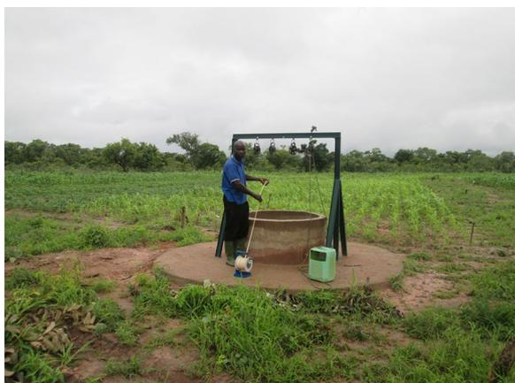
**Fig. 5** Water level measurement using Dip meters in Flola Technology Park (TP) located in Bougouni district. Photo Credit Birhanu Zemadim, 2015. A TP is a research site developed by Africa RISING program in Bougounia and Koutiala districts to conduct experiments for research and demonstrate new technologies to the farming communities
