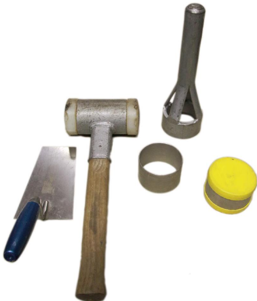
Figure 4.10: Sampling equipment including sampling ring, plastic caps, ram and hammer for installation, and shovel for excavation (photo: C. Schürz)
