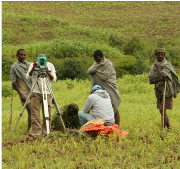
Figure 4.15: Land survey using the total station (photo: C. Schürz).
