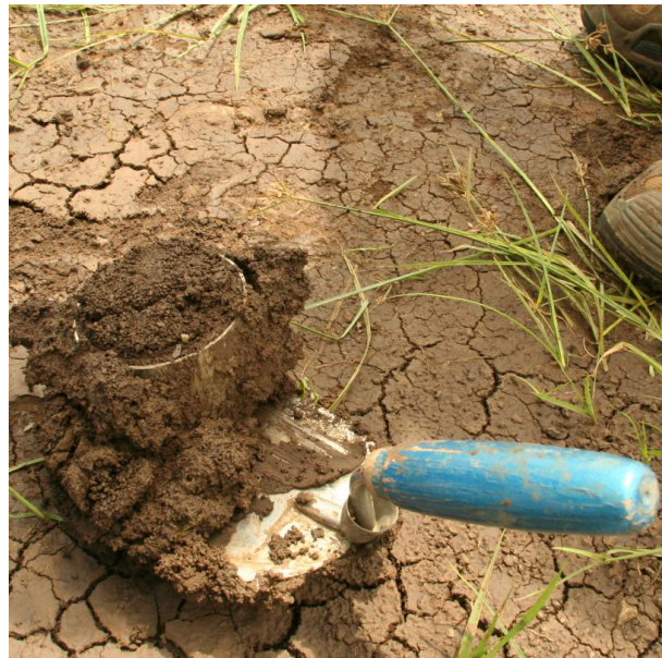
Figure 4.11: Taking undisturbed soil samples in the field. Extracted sampling ring with soil sample and excess soil (photo: C. Schürz).
