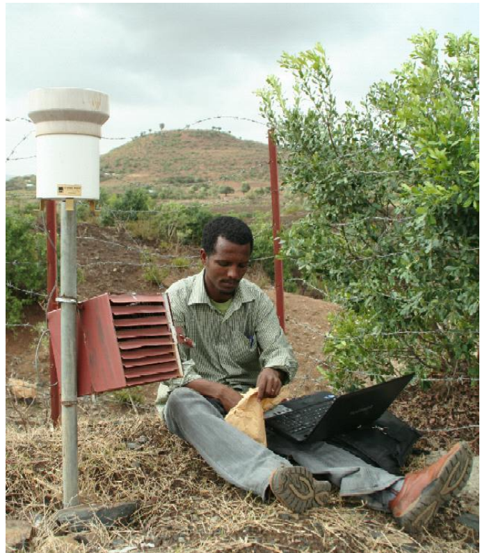
Figure 4.18: Reading out the rain gauge in the Aba-K'aloys sub-catchment (photo: C. Schürz).
