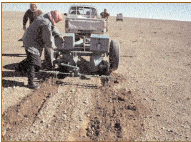
Left: Pitting-Seeder for range reseeding, (a modified Camel Pitter from Kimberly Seed Co.)
