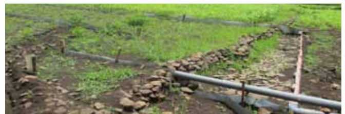
Photo 1: Measurement infrastructure to quantify and monitor the impact of soil conservation structures (stone bunds) on soil erosion (Photo credit: Claudio Zucca)
