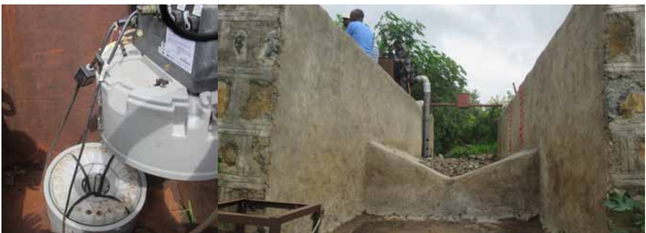
Photo 3: Automatic equipment to measure soil and nutrient losses located at the outlets of treated and untreated sub-watershed (Photo credit: Claudio Zucca)
