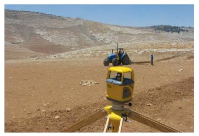
Laser guidance system for tractors: this innovation has greatly increased the speed and accuracy of preparing contour ridges
