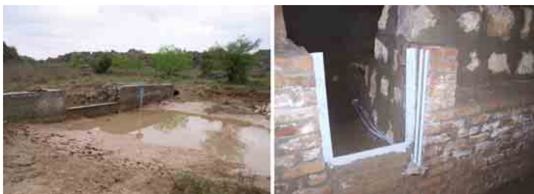
Weir with water level-recorder and vertical pipes for sediments sampling
