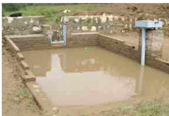
Stilling basin and water-level recorder for measurement of runoff and sediment
