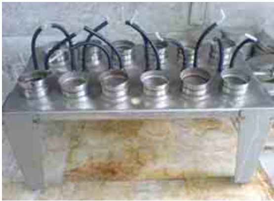
Figure 5.15. Equipment to determine the saturated hydraulic conductivity using the falling head method
