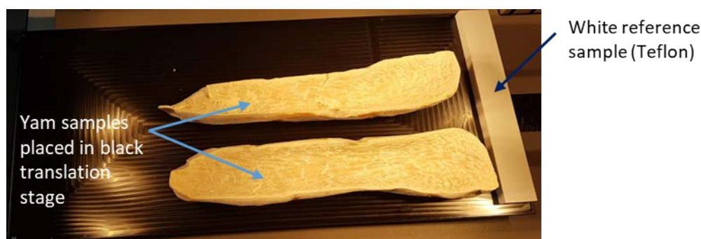
Figure 3: Black translation stage and a white reference sample (Teflon).
