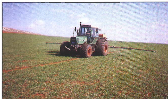
Low ground-pressure tires used for seed bed preparation and fertilizer top dressing. Pressure: 0.35 bar instead of the standard 1.6 bars.
