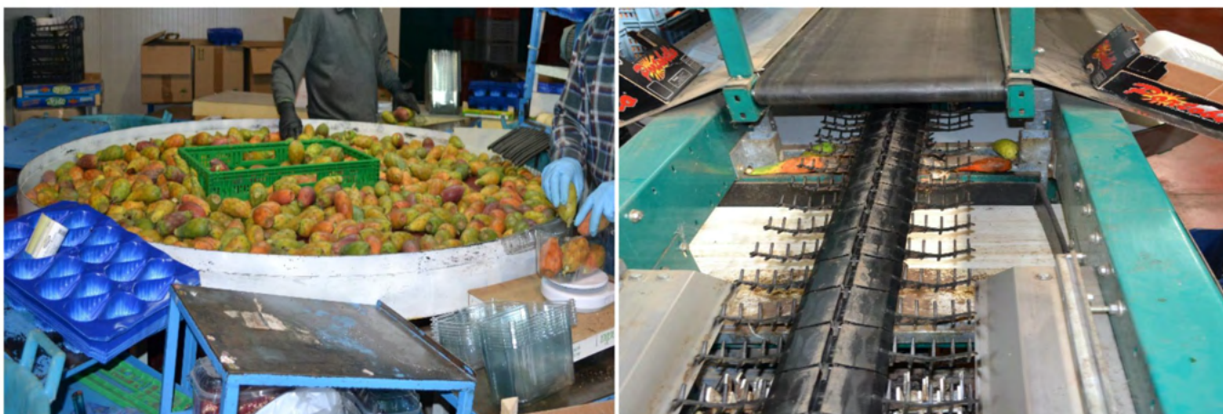
Figure 12 – Calibration, sorting and packing done manually on a rotating table (left); calibration through a packing line (right).
