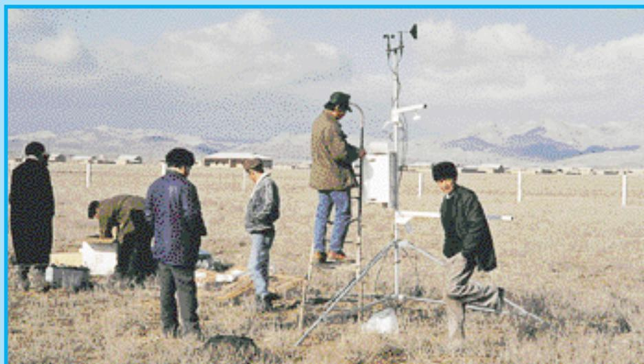
*Installation of a carbon-dioxide Bowen Ratio Equipment at a site near Samarkand in Uzbekistan. The equipment will be used for carbon-dioxide flux monitoring.*
