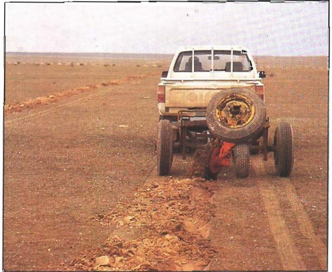
This simple pitting machine, developed at ICARDA, is useful in revegetation operations on degraded rangelands. The pits or holes made by it trap rainwater, organic matter, and seeds.
