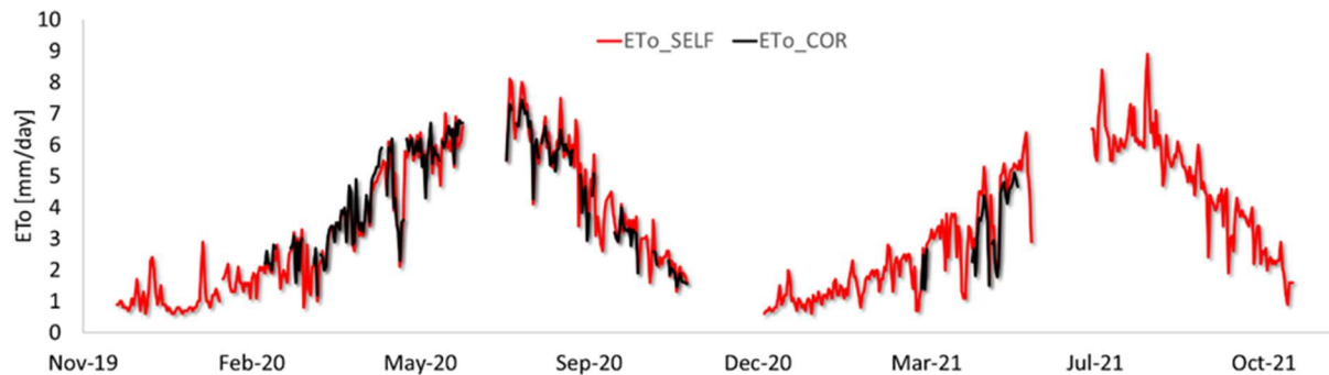
Figure 36 ETo determined at the El Khoudia Site, Tunisia, by CORDOVA-ET Station (ETo_COR) and on-site approach (ETo_SELF)
