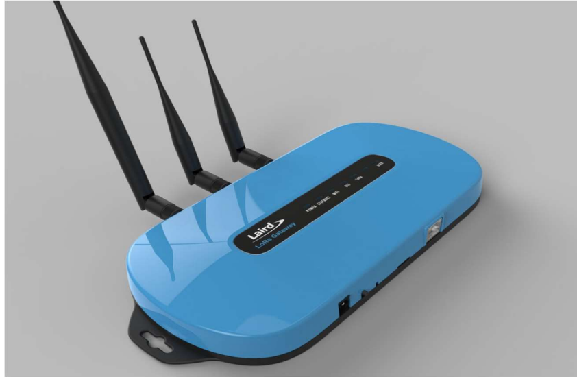
Figure 59: LoRaWAN gateway (Laird Sentrius RG186) used in the base stations. The long antenna receives the LoRaWAN data while the two smaller antennas are for the WiFi.
