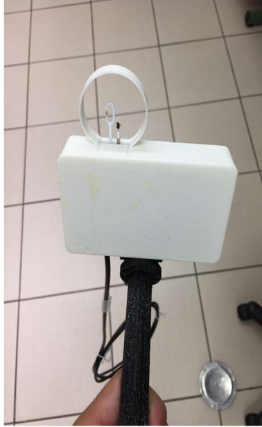
Figure 53: Test prototype for the CORDOVA wind speed sensor. A ring protective ring was added to protect the sensor from birds and any accidental damage. The box contains the electronics for powering and sensing.
