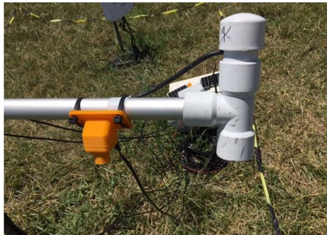
Figure 56: Infrared thermometer (Melexis MLX90614) in an orange 3D printed housing installed next to an IRTS-P Apogee sensor.
