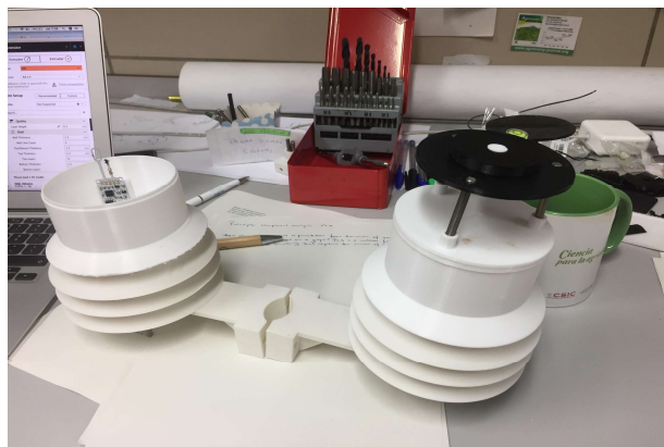
Figure 47. 3D printed radiation shields and sensor boxes containing the air temperature, humidity and barometer, hot wire anemometer and solar radiation sensor (on the right).
