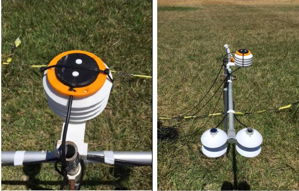
Figure 50: (a) Top view of the spectral sensor in the enclosure with the optic diffuser. In this test model, two sensors can be installed for simultaneous observation or for including visible and near infrared versions of the spectral sensor. (b) pyranometer and net radiometer (NR-01, Hukseflux, The Netherlands) used for the calibration.
