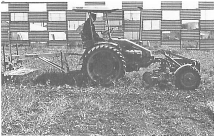
Fig. 1. Tool carrier tractor: front, mounted interrow cultivator; rear, 'weed wiper.'
