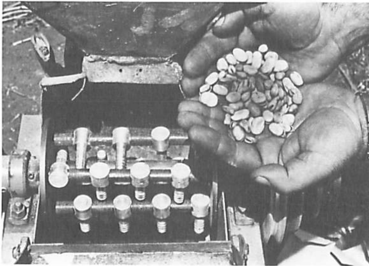
Fig. 2. Single-plant thresher with a flail-finger drum, interchangeable with standard rasp-bars or rigid-finger drums.
