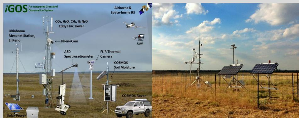
Fig. 1. Left: the schematic vision of Integrated Grassland Observation Site, and Right: flux tower system installed in El Reno, OK, USA. Each site is equipped with an Eddy covariance system for measuring fluxes, a PhenoCam to track vegetation phenology, and a COSMOS instrument to measure integrated soil moisture at the landscape scale.
