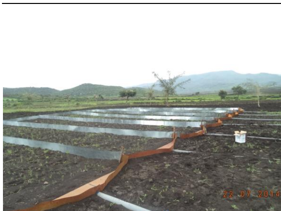
Runoff plots experimental setup, Worku Terfo field, Gumara- Maksegnit watershed Left: July 2014 | Photo by N. Demelash. Right: August 2015 | Photo by C. Zucca
