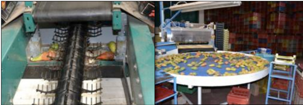
Figure 20: Sorting table at the end of a small and simple packing line (left). Processing lines used for citrus fruit are adapted to also process cactus pears, this occurs frequently in large packinghouses (right).
