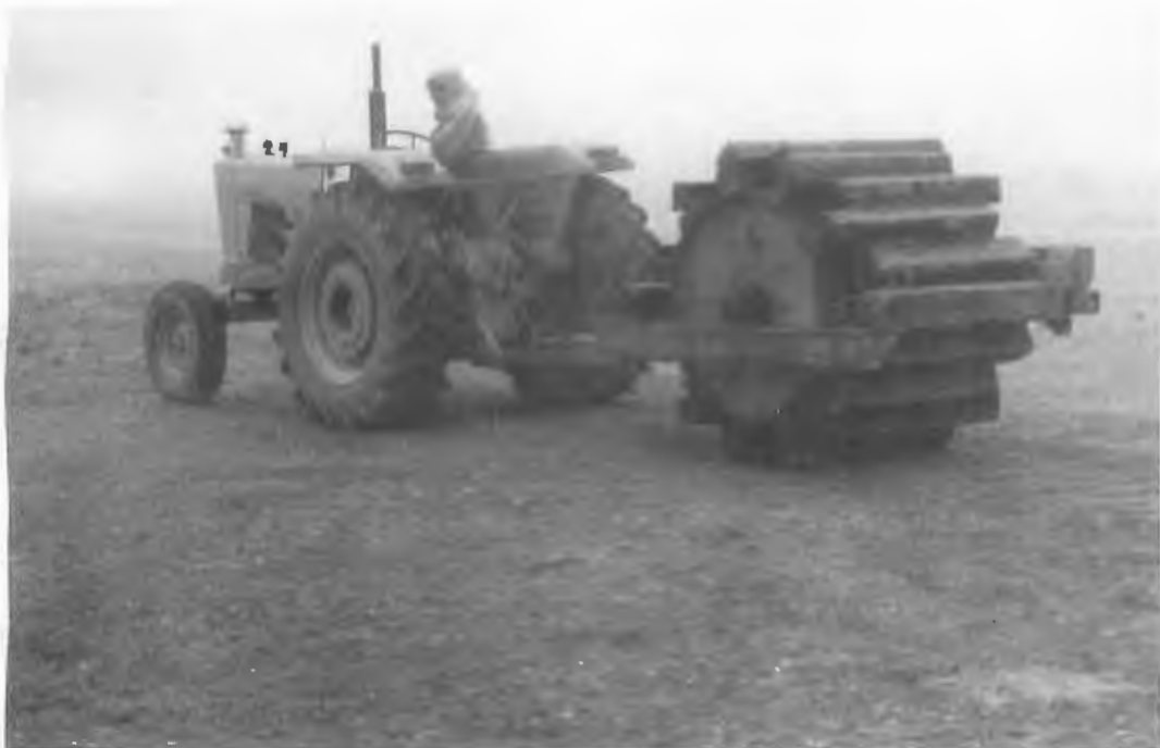
Photo 2. Land imprinter built at the ICARDA Station Operation Workshop with the support of Dr. J. Diekman. A new machine from an old story for rangeland rehabilitation
