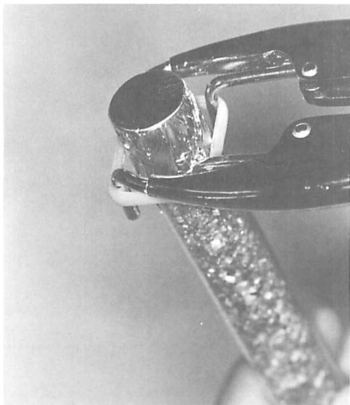
Fig. B.3.4. Placing Elastrator ring over foil cover on tube with special pliers.
