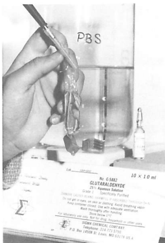
Fig. C.4.17. Adding 25% glutaraldehyde to the enzyme-antibody mixture in the dialysis bag.
