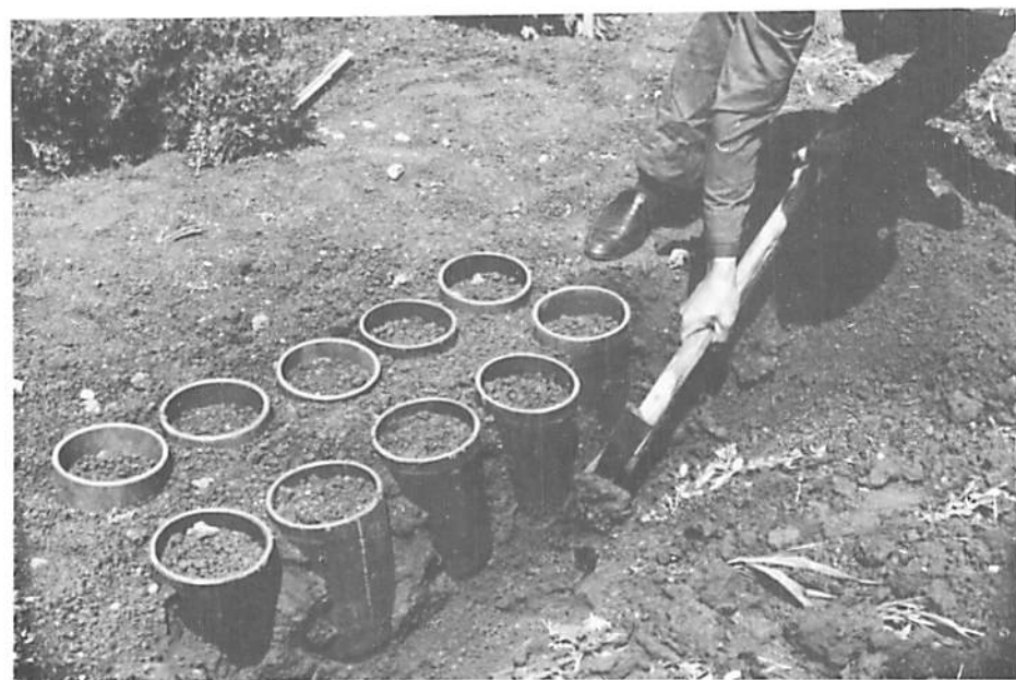
Fig. D.3.6. Digging trench along the line of inserted soil cores for easy removal of cylinders.
