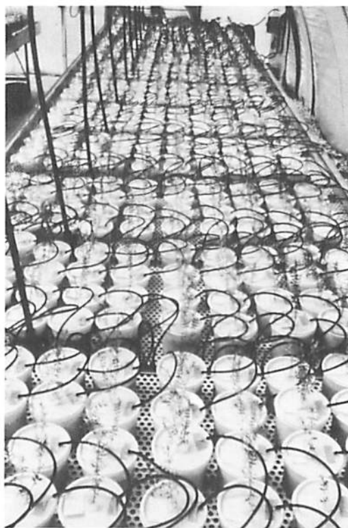
Fig. G.3.1. Aseptic hydroponic system used at ICARDA to evaluate symbiotic effectiveness.
