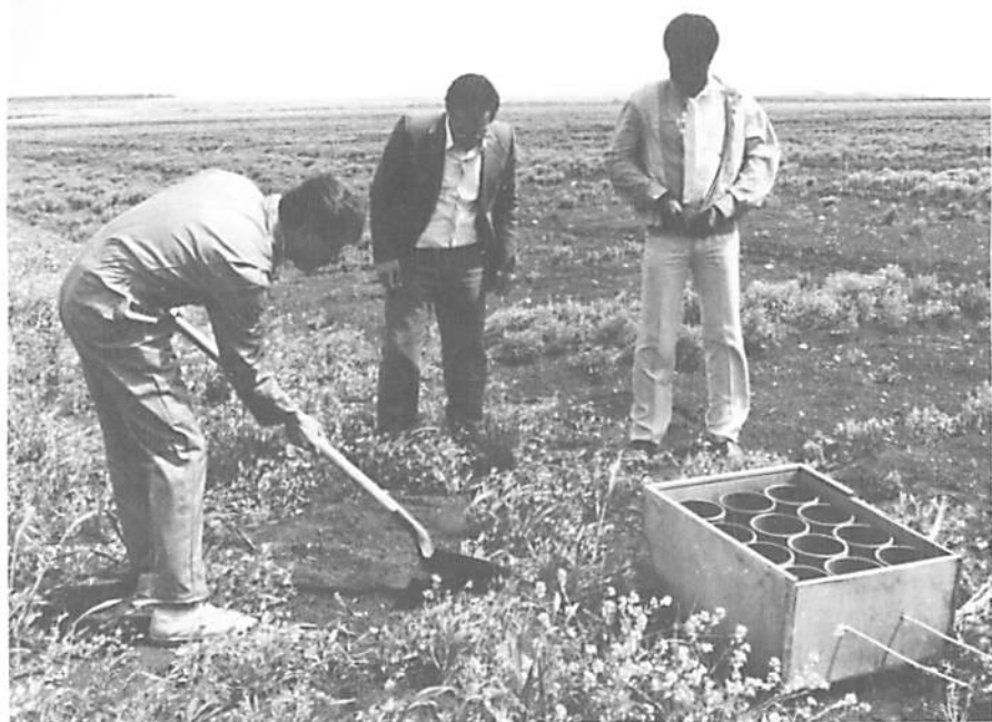
Fig. D.3.2. Clear the soil surface of rock, plants and debris before inserting cores.
