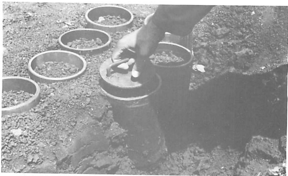
Fig. D.3.7. Placing the pipe disk over the surface soil in each core before removing from the ground.
