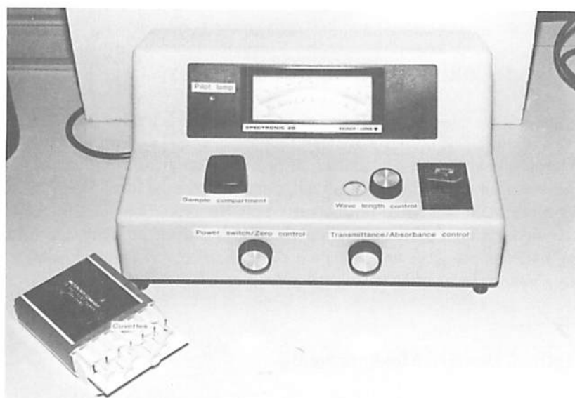
Fig. B.2.1. Spectrophotometer with components labelled.
