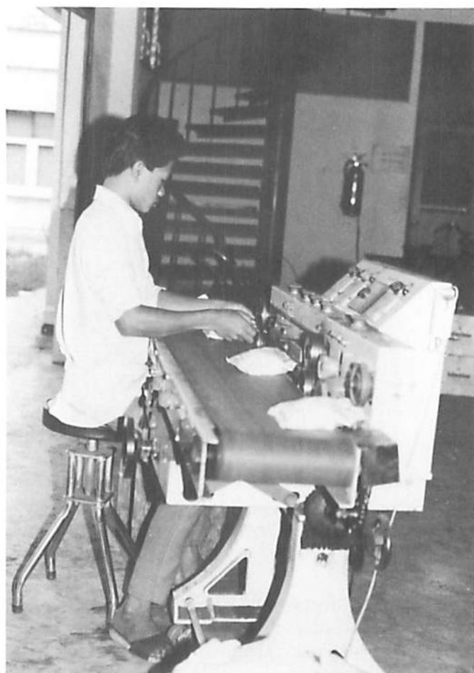
Fig. E.3.9. Commercial bag sealer used for large scale non-sterile inoculant production in Thailand.
