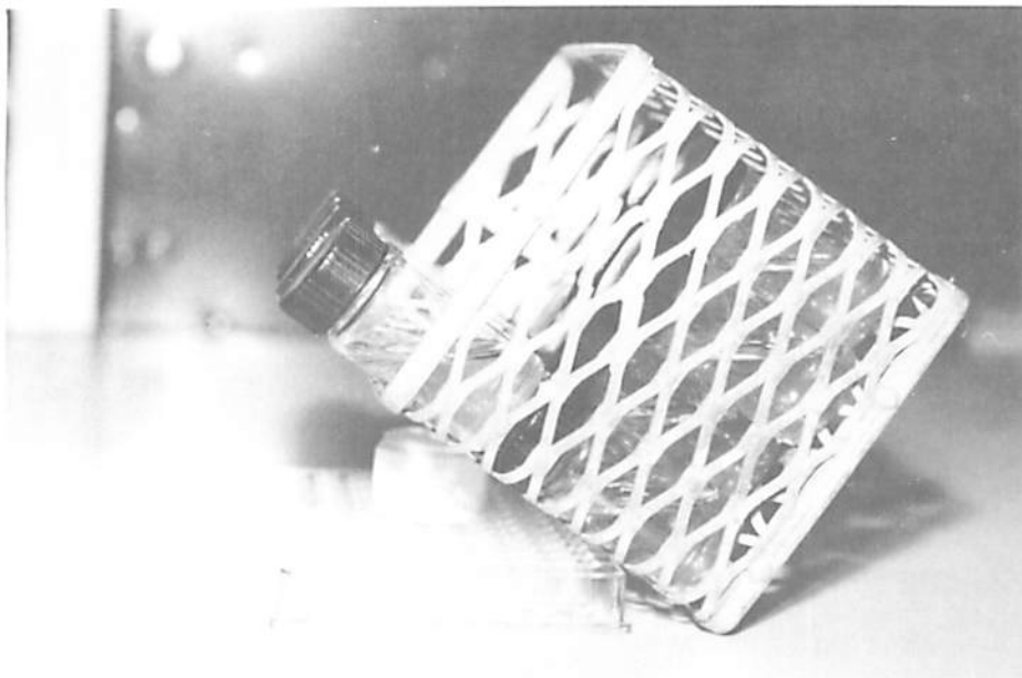
Fig. A.5.2. Cooling autoclaved tubes with melted YMA in a slant position.
