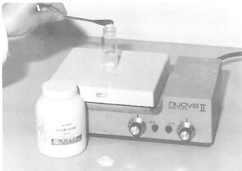
Fig. C.4.15. Reconcentration of fractions by slow mixing with sodium sulfate on a magnetic stirrer.
