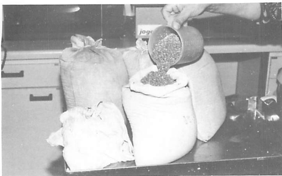
Fig. D.2.11. Filling cloth bags with moist washed substrate (vermiculite and gravel) prior to autoclaving.
