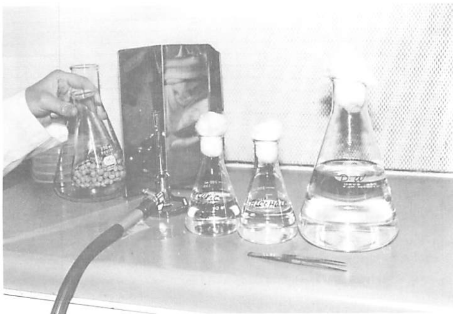
Fig. B.3.17. Sterilization of large legume seed. Seeds are left in the flask, with sterilizing and rinsing solutions added, mixed, and poured off in turn.
