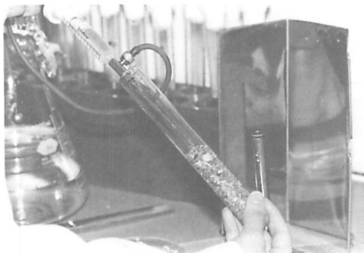
Fig. B.3.24. Watering tube with auto-filling syringe after planting seedling.
