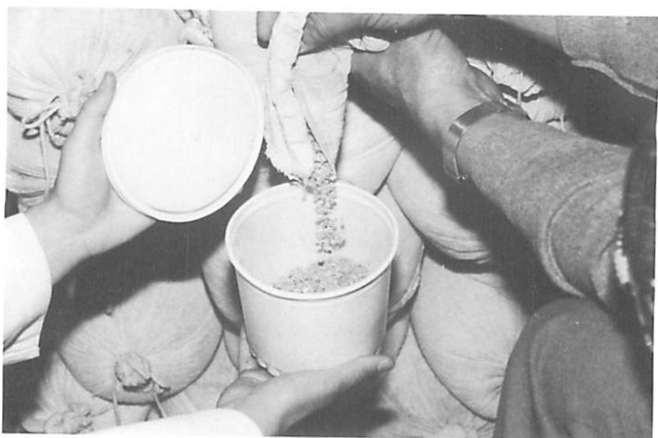
Fig. D.2.13. Transfer of sterilized gravel-vermiculite medium to sterile cup.
