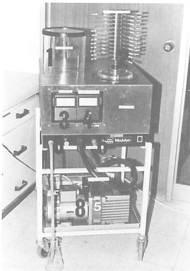
Fig. A.5.9. Lyophilizer machine with: 1) bell jar; 2) ampule manifold; 3) vacuum gauge; 4) temperature gauge; 5) drain valve control; 6) air admittance valve; 7) vacuum line; and 8) vacuum pump.
