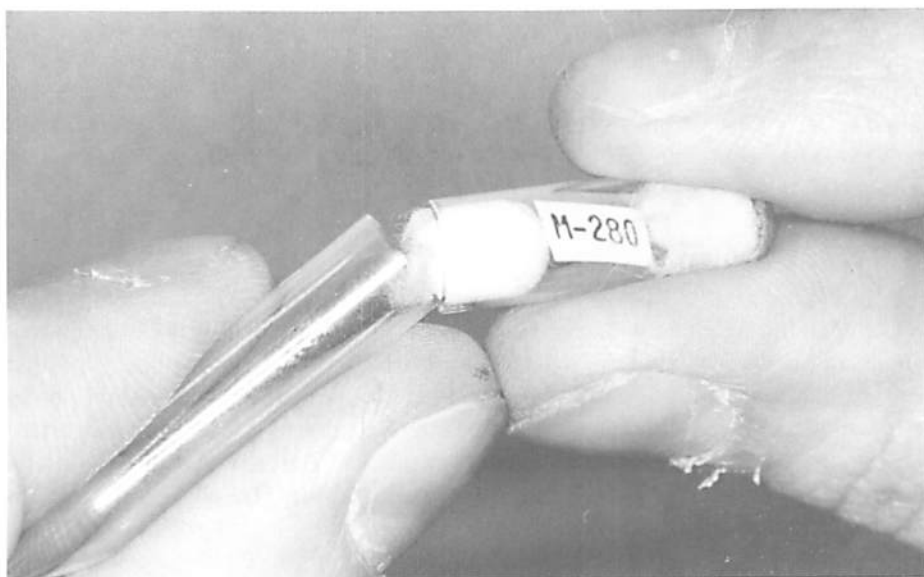
Fig. A.5.21. Breaking open an ampule under laminar flow hood.
