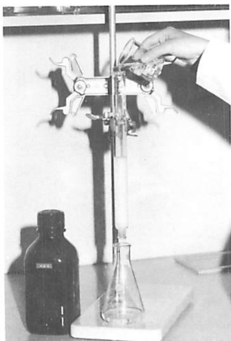
Fig. C.5.24. The column is equilibrated by adding 3 column volumes of PBS with merthiolate.
