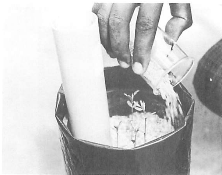
Fig. D3.19. Covering surface of core with heat-sterilized gravel to prevent surface contamination.
