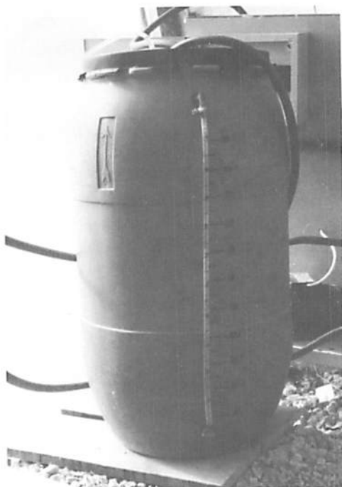
Fig. D.2.14 N-free nutrient solution reservoir with clear tubing volume gauge.
