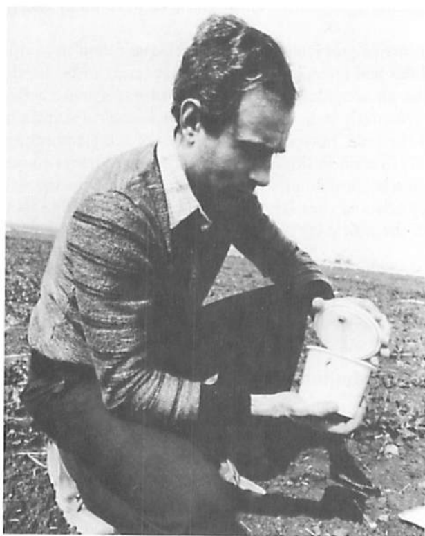
Fig. H.1.2. Airtight plastic container with subseal port in the removable lid for injection and removal of gas.
