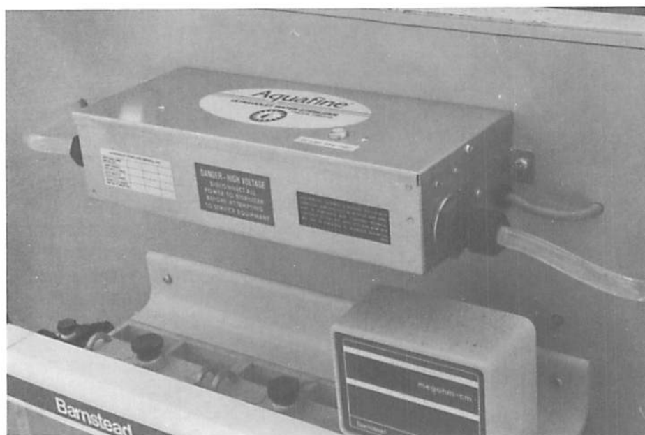
Fig. D.2.18. Ultraviolet light unit to sterilize deionized water flowing into reservoir.
