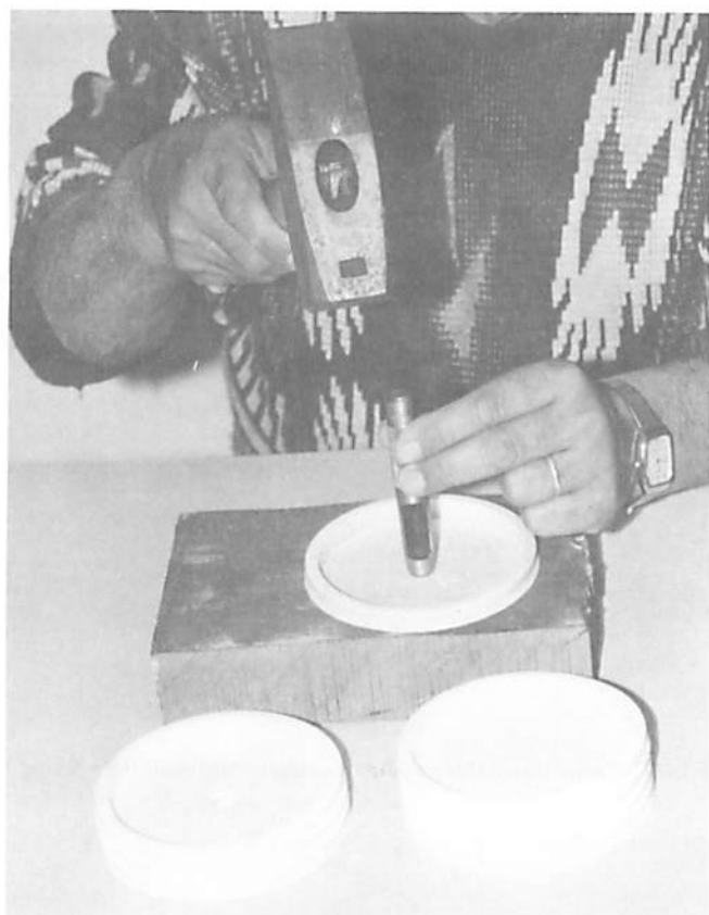
Fig. D.2.10. Using a punch to make plant growth hole in cup lid.
