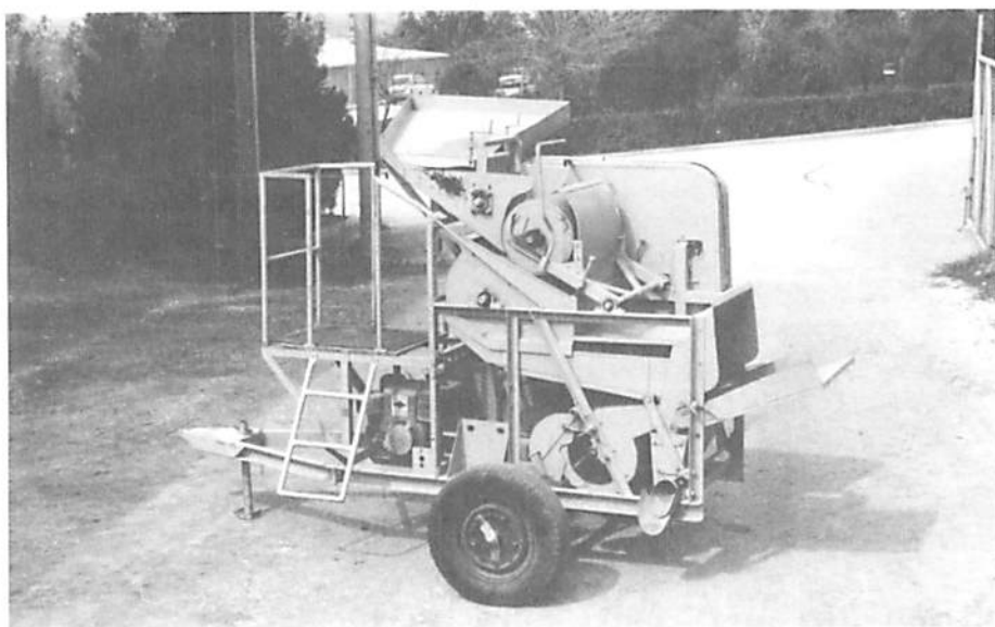
Fig. F.7.3. A small mechanical thresher can be used if a large quantity of plant material is harvested.
