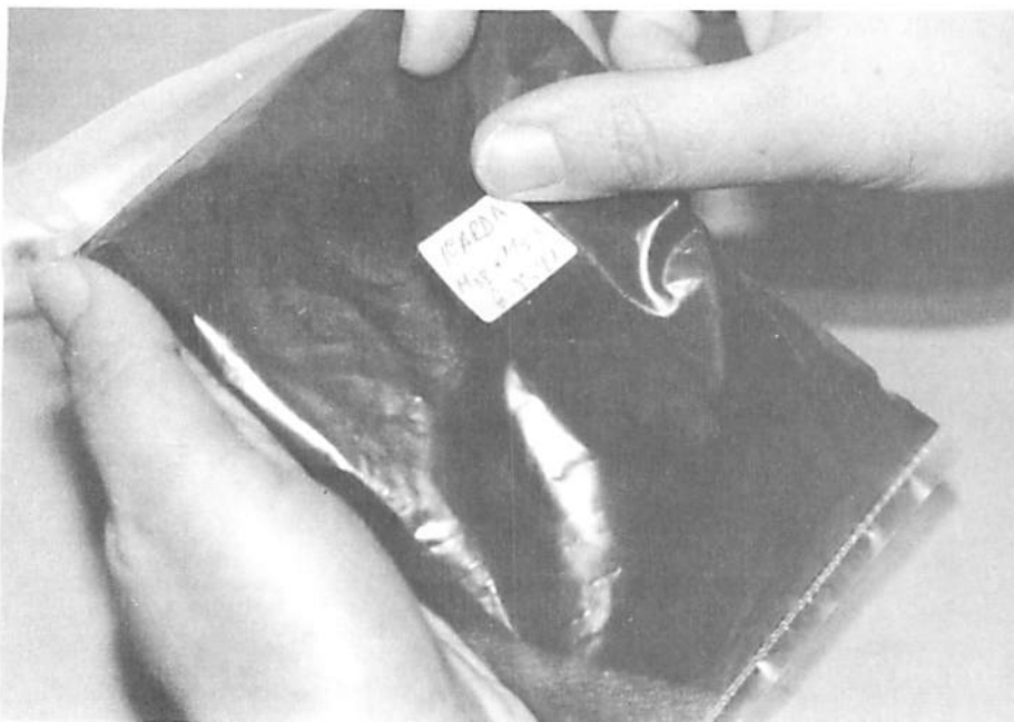
Fig. E.3.6. The puncture hole is wiped immediately after injection with 90% alcohol, then the hole is covered with a self-sticking label to prevent contamination and label the bag contents.
