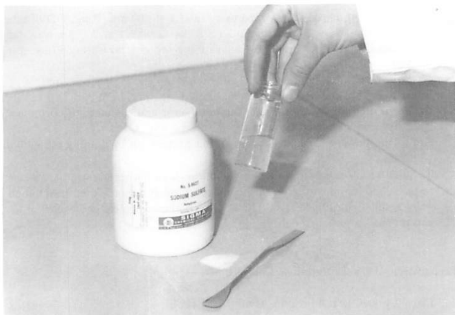
Fig. C.4.6. Manual stirring for 5 minutes during addition of sodium sulfate.
