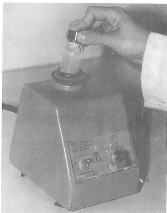
Fig. C.3.1. Suspending a rhizobial slant culture using a vortex mixer.
