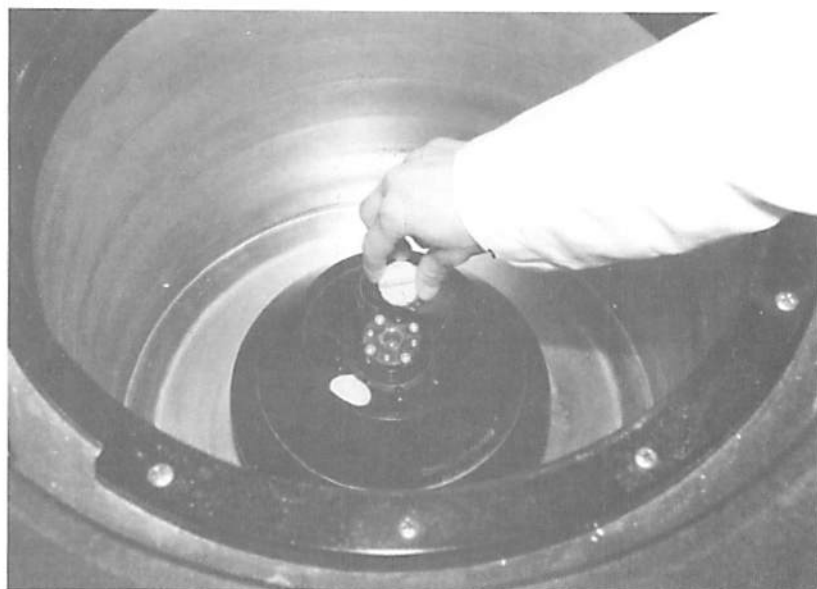
Fig. C.3.5. Using a refrigerated centrifuge to obtain a pure-cell pellet.
