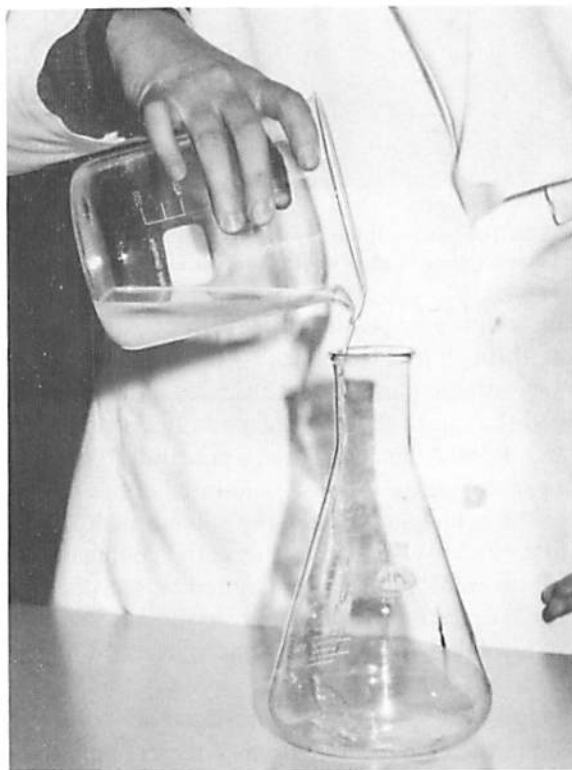
Fig. C.5.22. Once the Sephadex has settled, the fine particles are removed by decanting the supernatant.
