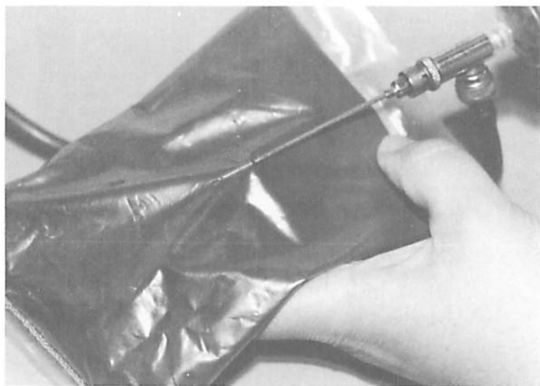
Fig. E.3.5. Insertion of needle nearly parallel to bag surface for injection of broth into carrier.
