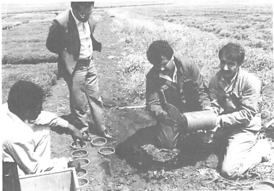
Fig. D.3.9. Trimming loose soil from bottom of soil core so that completed assembly will sit flat on table top.
