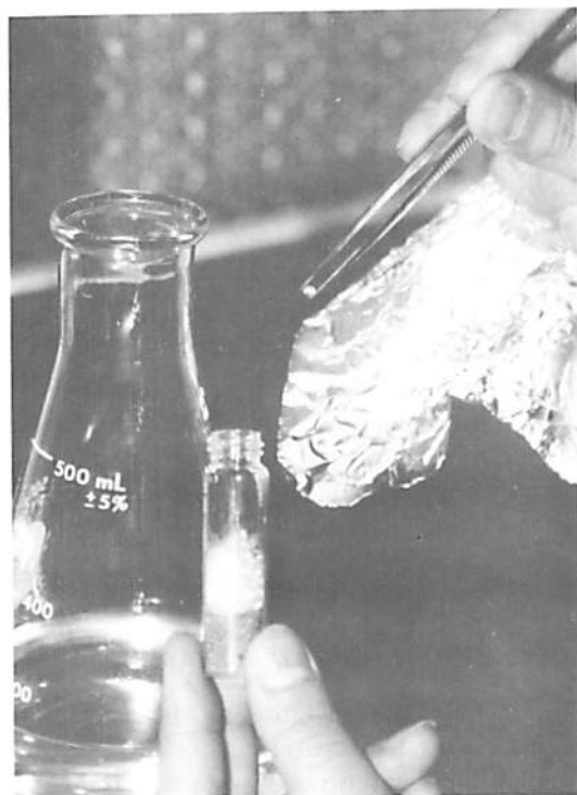
Fig. A.5.7. Transferring bead to flask containing broth.
