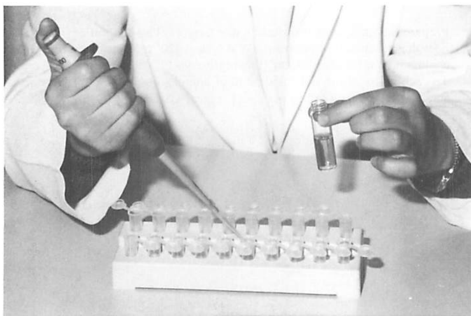
Fig. C.5.32. Distribution of purified FA conjugate in tubes for further storage in freezer at -20^{\circ}\text{C} .
