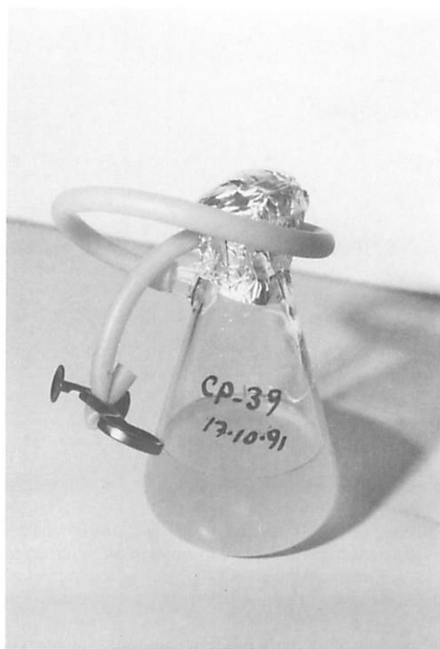
Fig. E.2.10. Starter culture in side-arm Erlenmeyer flask for inoculation of 100 L fermentor.
