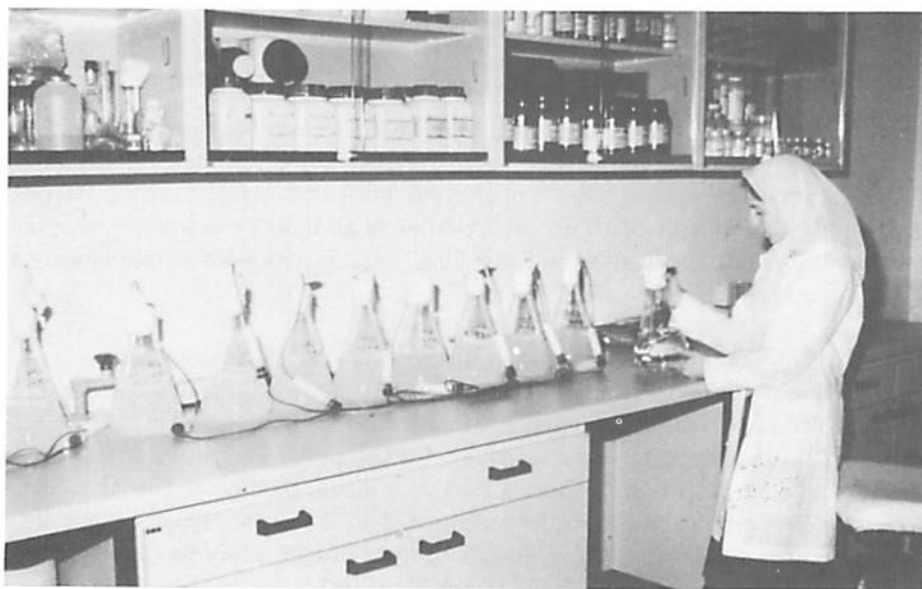
Fig. E.2.1. About 15 L of liquid media can be aerated by a small aquarium pump.
