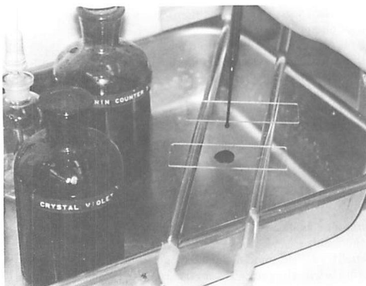
Fig. A.6.2. Simple staining rack holding slides over tray.
