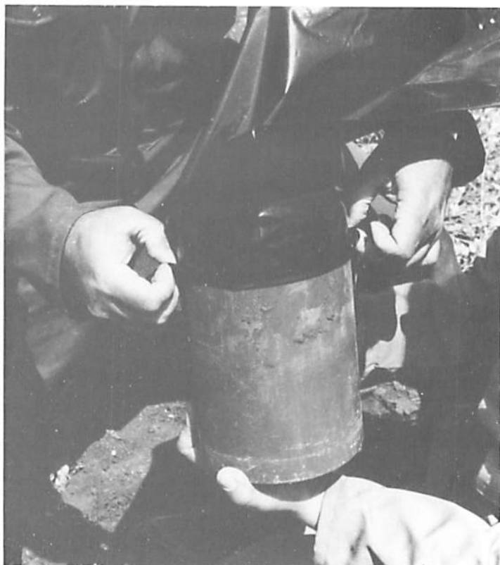
Fig. D.3.10. Applying a tight-fitting plastic bag over the bottom of the core.
