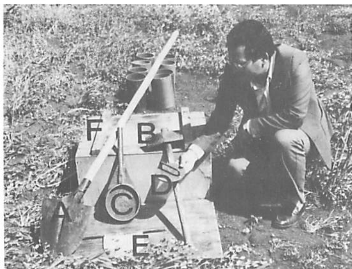
Fig. D.3.4. Tools for soil core collection including: A) shovel; B) sledge hammer; C) impact cap with handle; D) pipe disk; E) removal shovel, and F) box for core transport.
