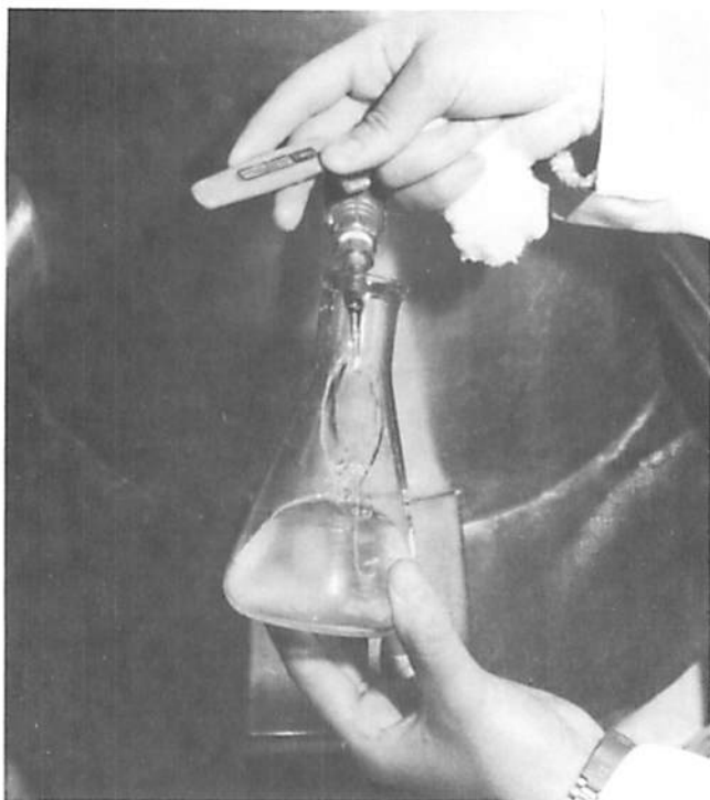
Fig. E.2.12 Collecting sample from fermentor for purity check. Sampling port should be flamed thoroughly before and after sample collection to prevent contamination of fermentor contents.
