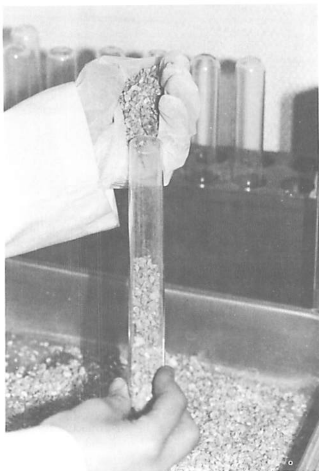
Fig. B.3.15. Filling tube system with dry gravel/vermiculite mixture prior to autoclaving.
