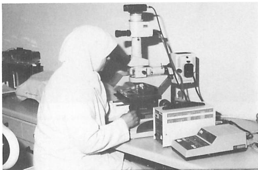
Fig. C.5.39. Observing prepared slide under a UV-capable microscope.
