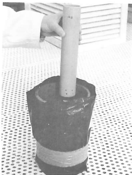
Fig. D.3.17. Irrigation tube for even distribution of water in soil core. Note that drainage holes are placed only on side of tube pointing toward core center, to prevent direct water loss down the side of the core.
