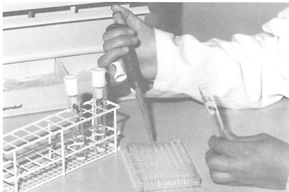
Fig. C.4.27. Fresh homologous and heterologous YEM slant cultures are diluted in PBS to an optical density of 0.4, then diluted 1:50 in water before adding to wells as controls.
