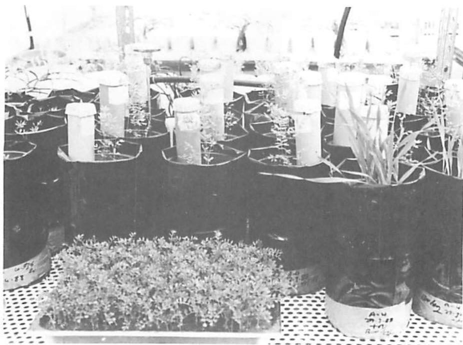
Fig. D.3.13. Drilled steel table surface to prevent cross-contamination between pots or cores.
