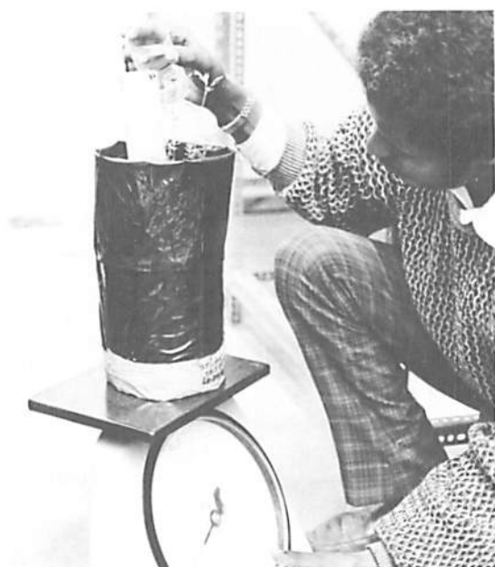
Fig. D.3.22. Cores are watered periodically to the field capacity weight indicated on the label to provide equal water availability to all treatments.
