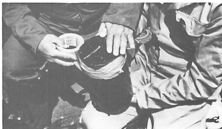
Fig. D.3.11. Duct tape is applied tightly around bottom of core to prevent loss of soil when core is set upright.
