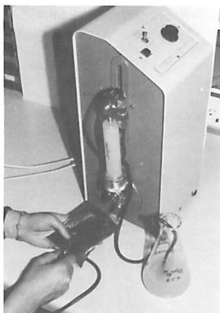
Fig. E.3.4. Automatic syringe used to inject a specific amount of liquid repeatedly. With this device, large numbers of peat packages can be injected with relative ease and good contamination control.
