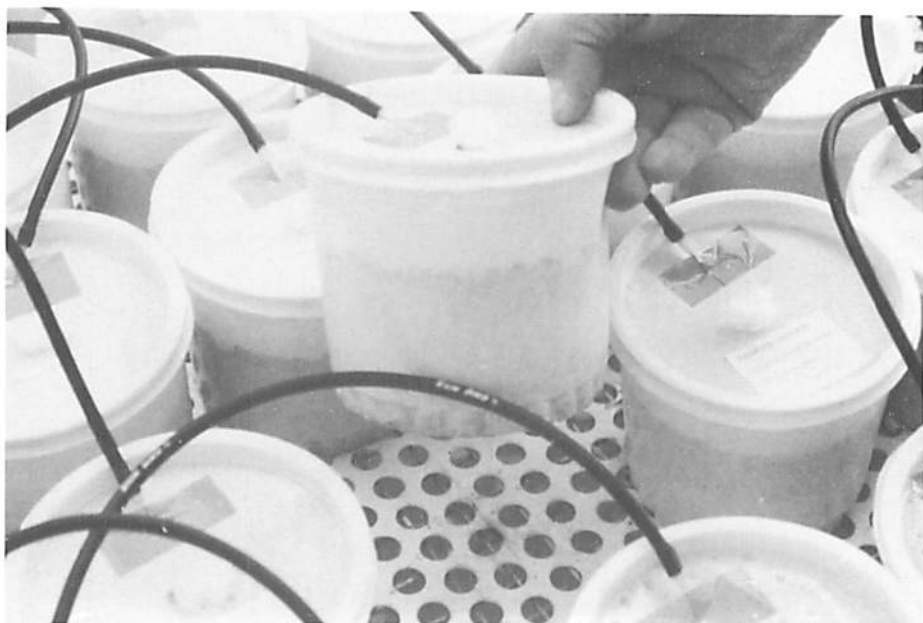
Fig. D.2.17. Drilled steel table surface allowing water to drain away from cups and prevent contamination.
