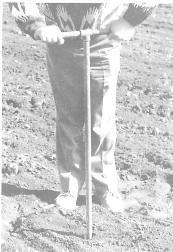
Fig. B.3.1. Soil sampling coring tool in use in the field (soil auger).
