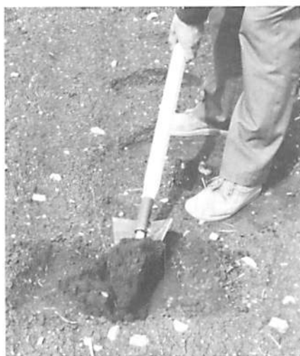
Fig. F.1.1. Long-nose trowel for the extraction of soil samples.
