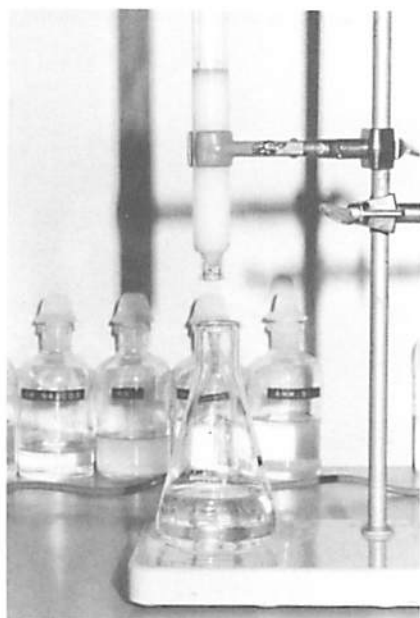
Fig. C.5.27. As the last of the conjugate penetrates the Sephadex surface, PBS is added.
