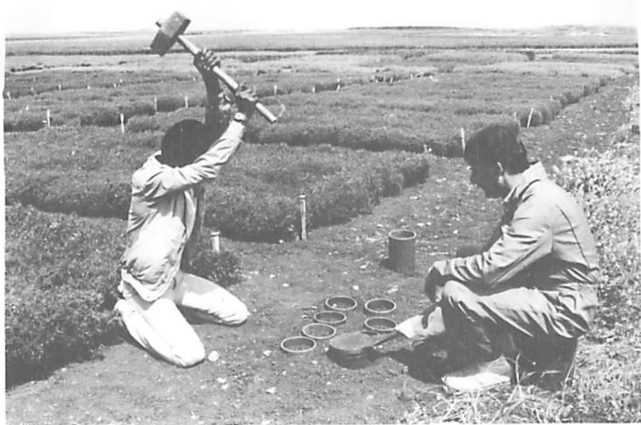
Fig. D.3.5. Pounding core cylinder into soil using an impact cap and a heavy sledge hammer. Two persons are required as cap must be held tightly on core so that the cylinder enters the soil vertically.
