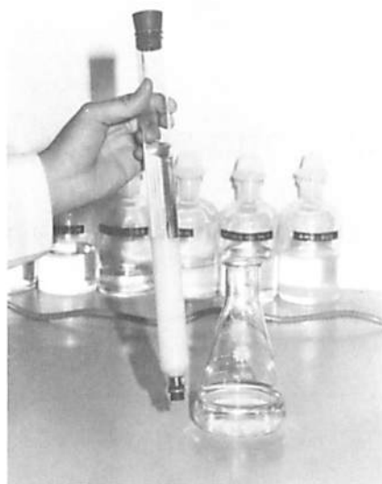
Fig. C.5.29. Cover the column with a rubber stopper after use and store in the refrigerator.
