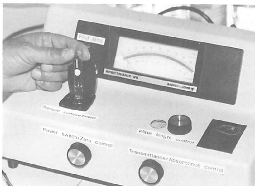
Fig. B.2.2. Cuvettes, of special optical glass, for use in spectrophotometer.
