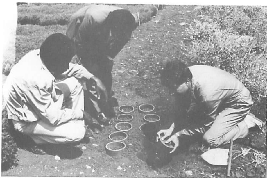
Fig. D.3.8. Removing soil core from moist soil by breaking core off into trench. In sandy or dry soil, the removal shovel (shown) is slipped carefully under the bottom of the core (to prevent soil loss from core) and the whole assembly is removed from the ground.
