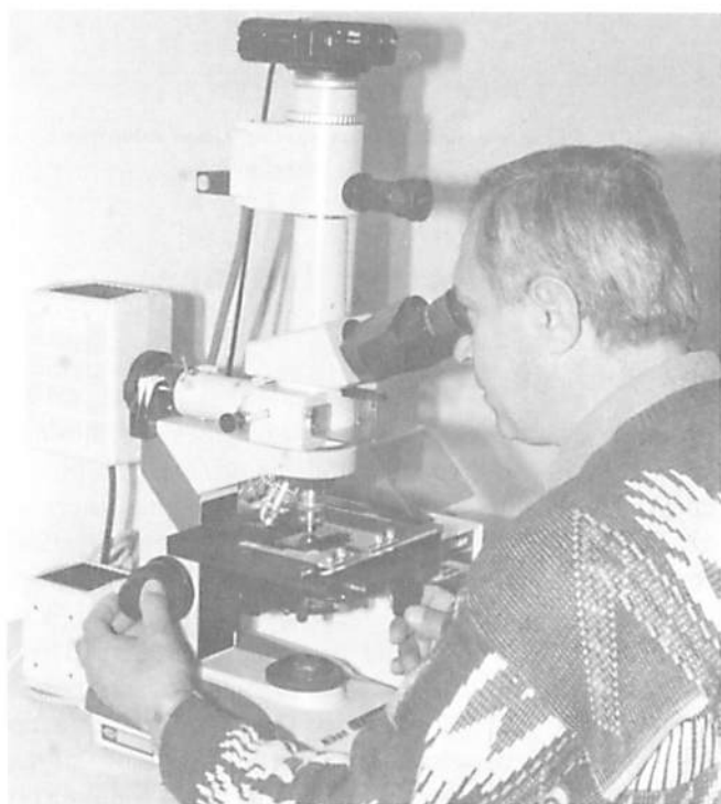
Fig. C.5.1. Fluorescence microscope, with fluorescent light source, UV filters, and camera attachment
