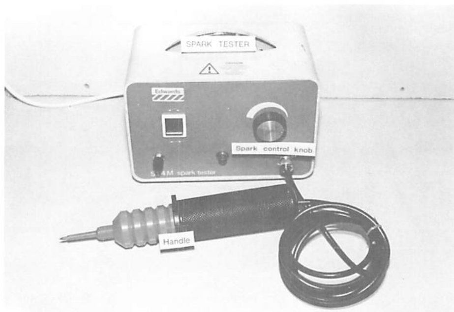
Fig. A.5.18. Spark tester showing essential parts.
