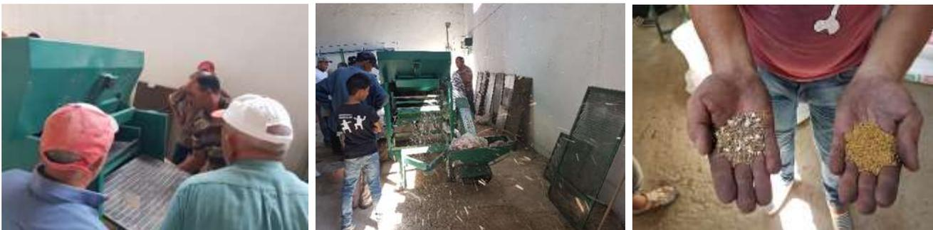
Figure 12: Changing sieves, cleaning unit in action, cleaned seeds (Udo Rudiger/ICARDA)
