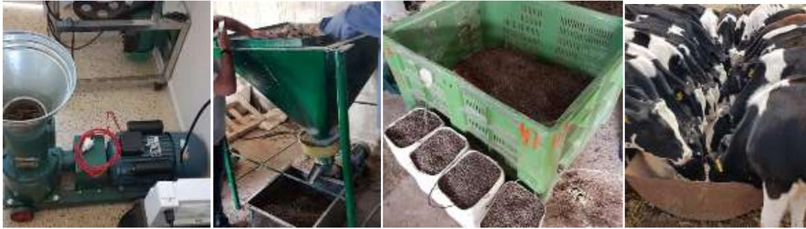
Figure 6: Pellets produced by imported pellet machine (Udo Rudiger/ICARDA)
