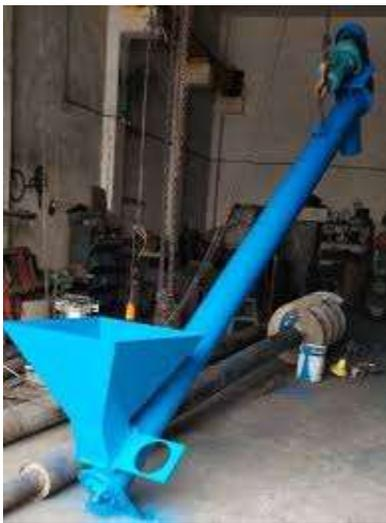
Figure 13: Conveyor screw for seed transportation
