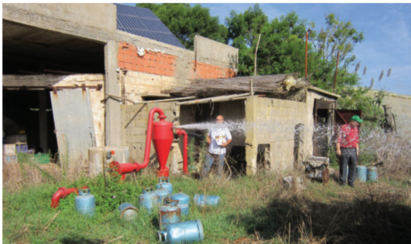
Using liquefied petroleum gas cylinders to extract groundwater for irrigation, Morocco
