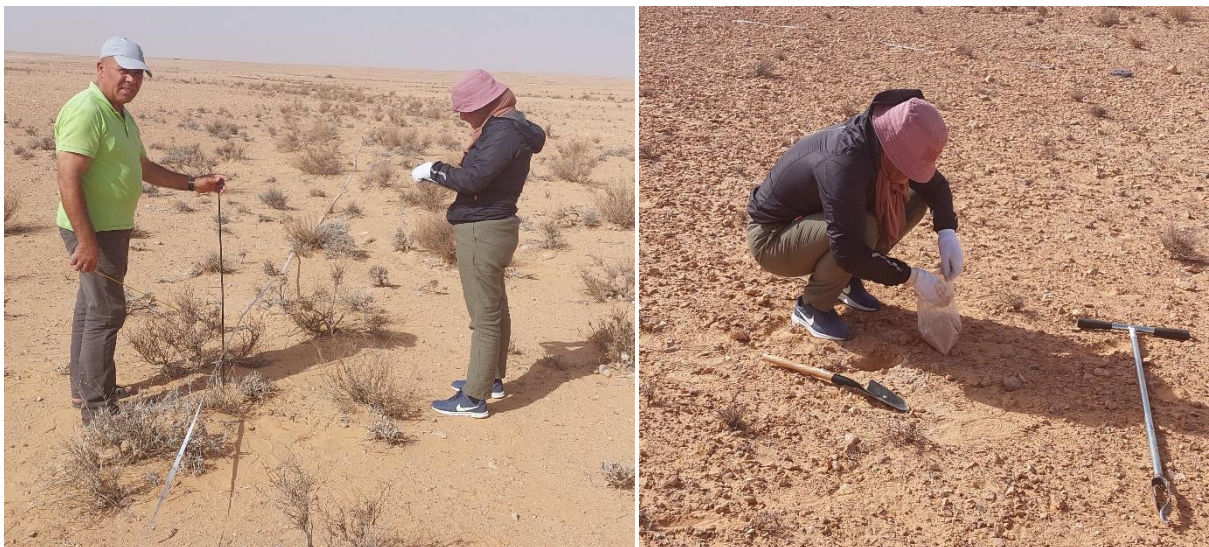
Figure 4. Participants Collecting Data Using the Line Point Intercept (LPI) Method Along with Soil Sampling.
