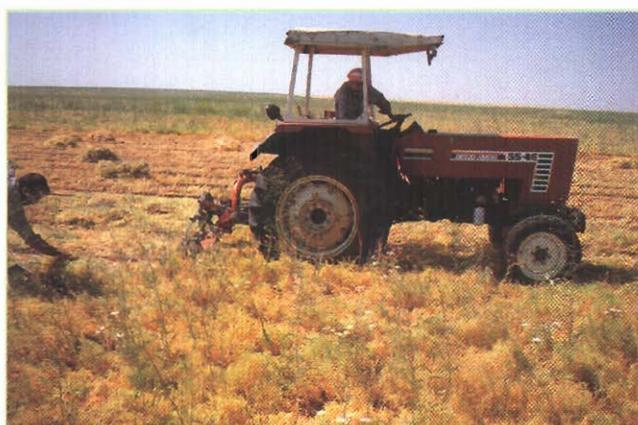
A side-mounted, tractor-operated, double-knife cutter bar in operation for harvesting lentil in Urfa, Turkey.
