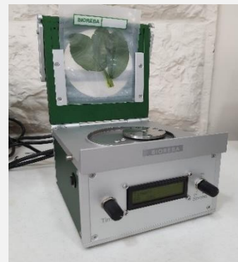
Samples extraction using HOMEX XS homogenizer
