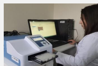
Measuring color intensity at 405 nm using ELISA microplate reader
