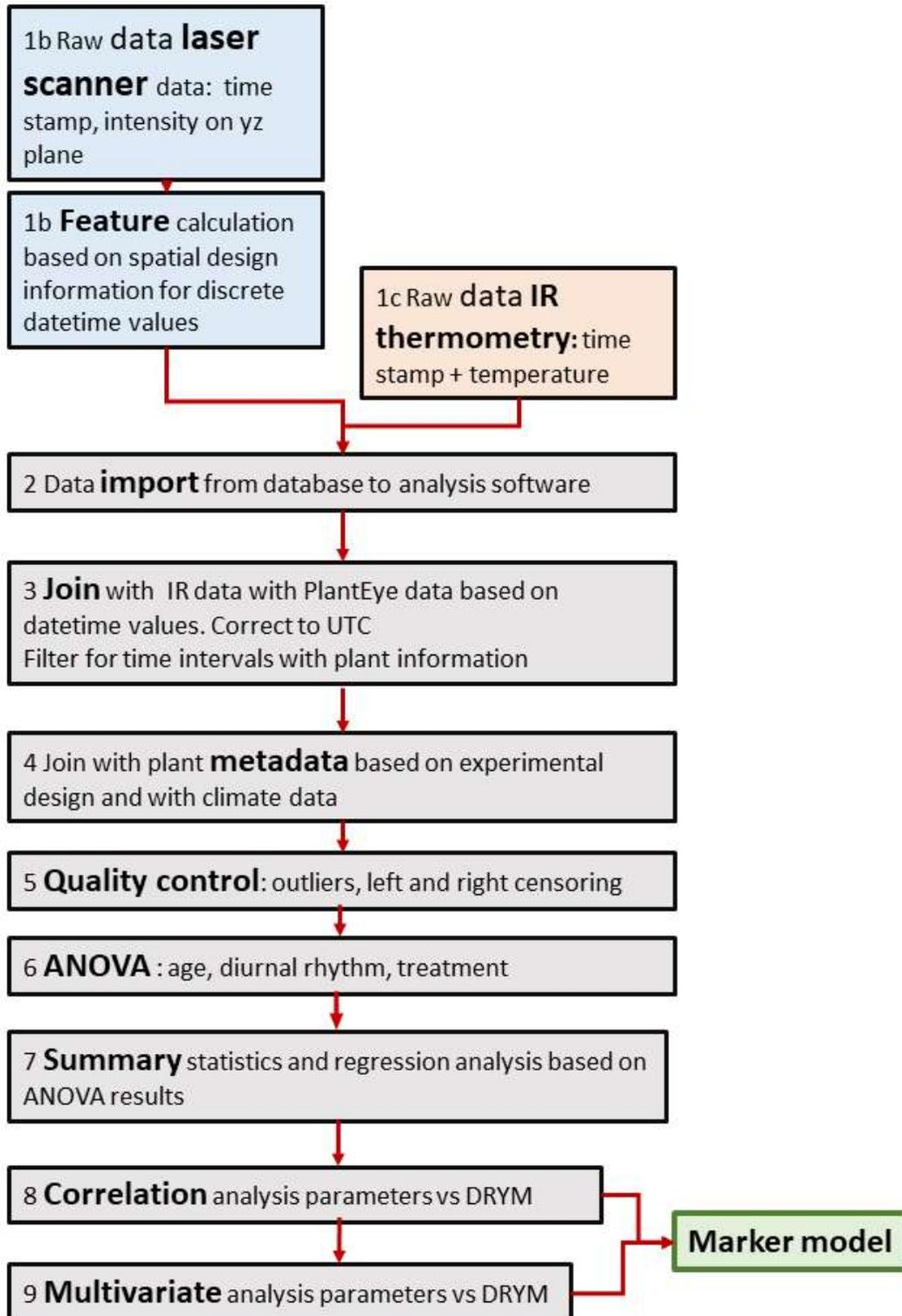
Figure 3. Data analysis workflow for laser-scanner and infrared-thermometry data.
