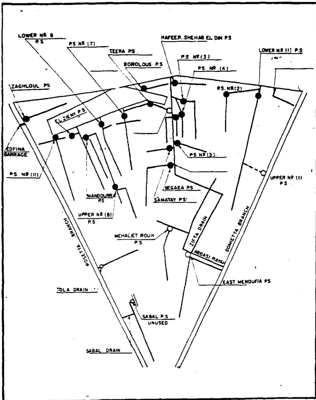
Fig. 8. Drainage system in the Middle Delta.
