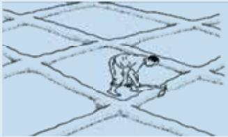
Designed to collect and hold rainfall as runoff water is channeled to the lowest point and stored in an infiltration pit. Usually 1–2 m long, with basins of up to 30 m. Ideal on deep soils (1.5–2 m), annual rainfall amounts of 150 mm and above on flat surfaces to slopes of 5%.
