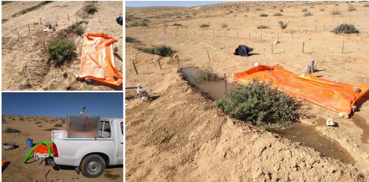
**Figure 7** The forced infiltration experiment performed in the field.
