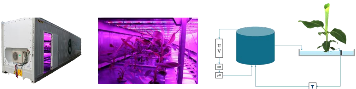
Figure 1: The 'bananaTainer' is a modified, climate controlled reefer container specifically designed to house 504 banana plants. The water circuit contains 2 loops, the main loop supplying the plants with water by an overflow system, passing a particle filter (80 micron) before returning to the nutrient tank. The secondary loop treats the water with a UV source and leads the water over an EC and pH sensor.
