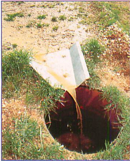
Where there is no local information available, runoff coefficient plots are essential to determine design parameters for micro-catchment systems.
