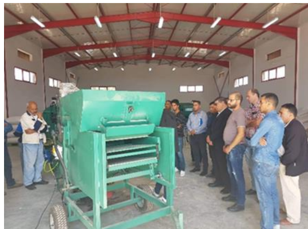
Fig 2: :Mobile seed cleaning and treatment unit (Photo: Zied Idoudi, ICARDA)
