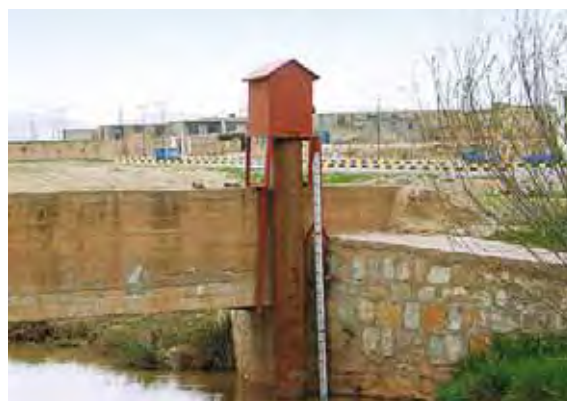
Figure 3.15. The data logger and a stage attached to the flume wall at Halashi station.
