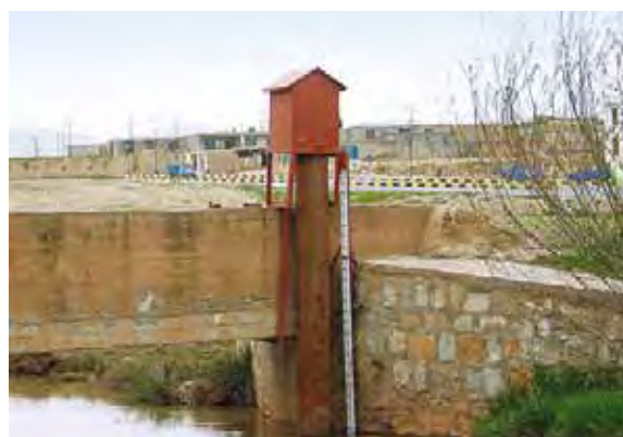
Figure 4.18. The data logger and a stage attached to the flume wall in Halashi station.
