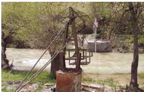
Figure 3.6. View of Honam hydrometric station with derricks and cable.
