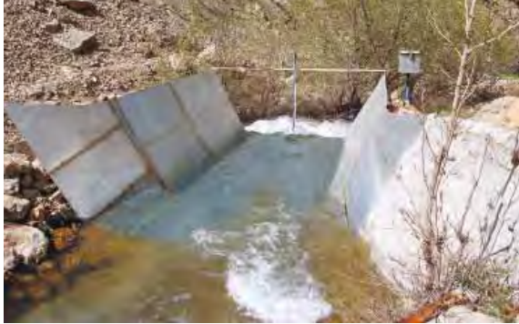
Figure 3.8. View of the supercritical flume installed in Presk spring.
