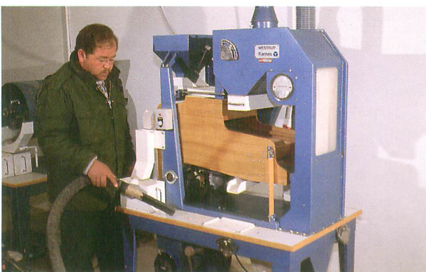
4.3 Air-screen cleaner with three layers
