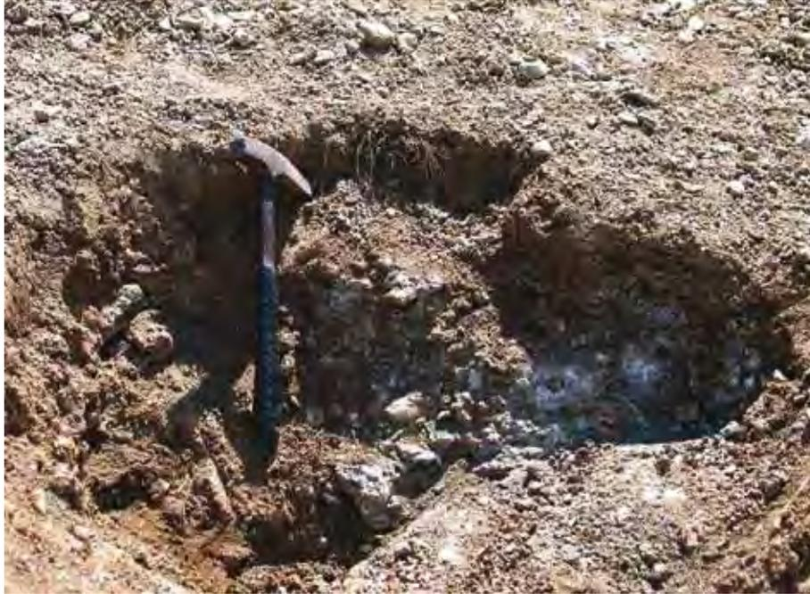
Plate B7. Fine-loamy, mixed, mesic Lithic Xerorthents (Map unit 35, Pedon 75) (M. Sepahvand, 2008).
