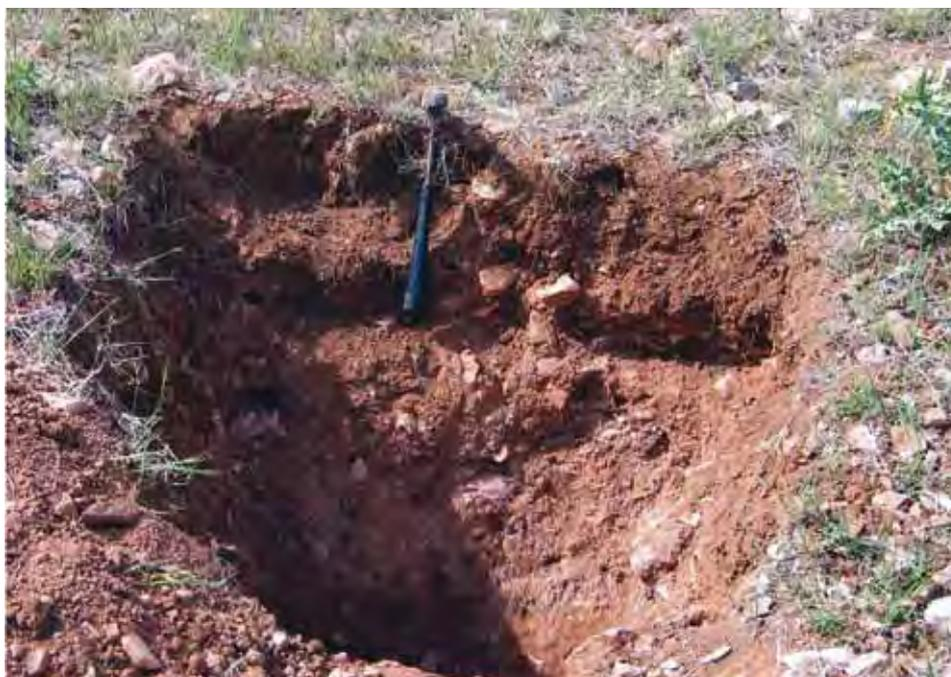
Plate B1. Fine, mixed, mesic Typic Calcixerepts (Map unit 1, Pedon 81) (M. Sepahvand, 2008).
