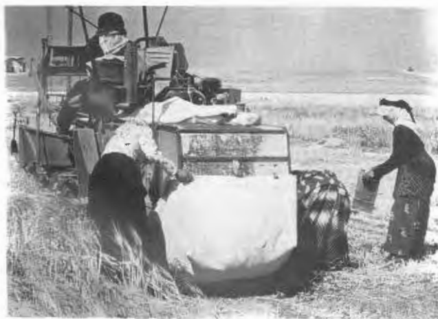
ICARDA straw collector mounted on a small plot combine is being used to assess cereal biological yield.
