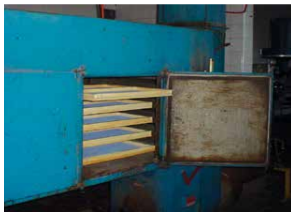
Forced-air drying tunnel used to obtain dehydrated sheets of cactus pear pulp
