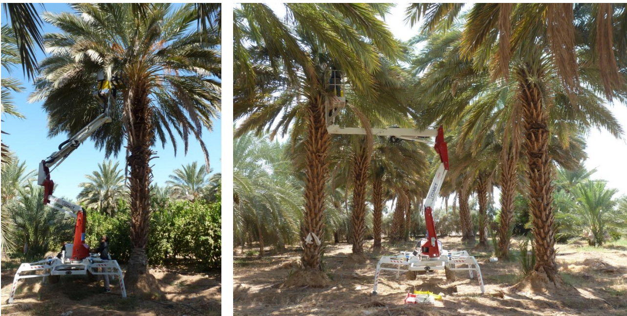
Figure 3.1 and 3.2. Placing for the two different methods: "360°", on the left, and "180°+180°" on the right.
