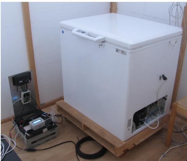
*Ice-maker with batterie, control unit(Socobox) and data logging*
