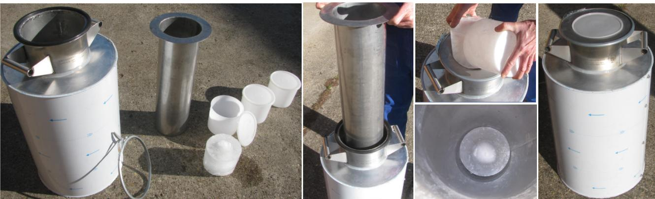
Prototype of the final version of the isolated milk can
