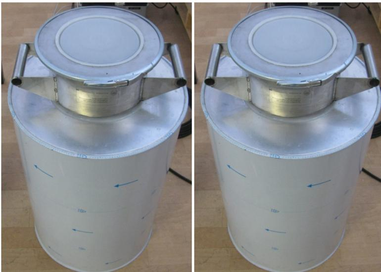
*Two milk cans per system for milk cooling of a total of 60 L/day*
