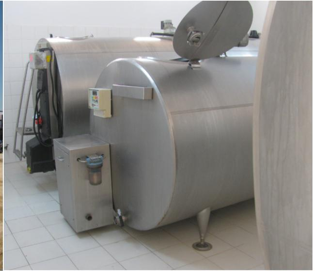
*Tanks for milk storage at 4°C*
