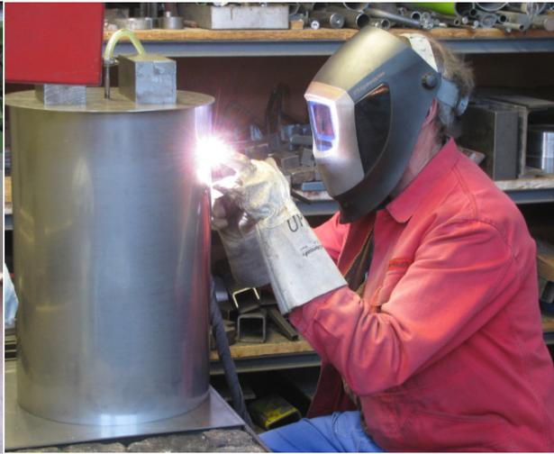
Electrical welding with shielding gas inside the milk-can
