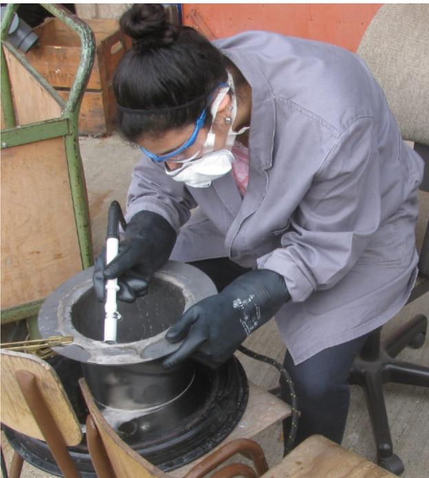
Electro-chemical cleaning of welding lines
