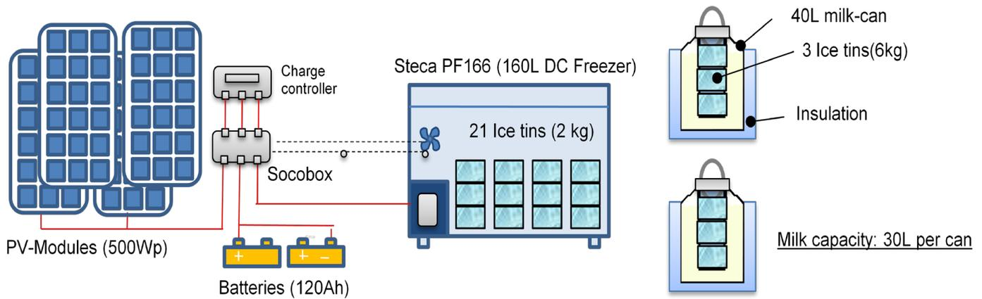
*System configuration of one single system (PV modules with structure, charge controller, socobox, DC-Freezer and 2 Isolated milk cans)*
