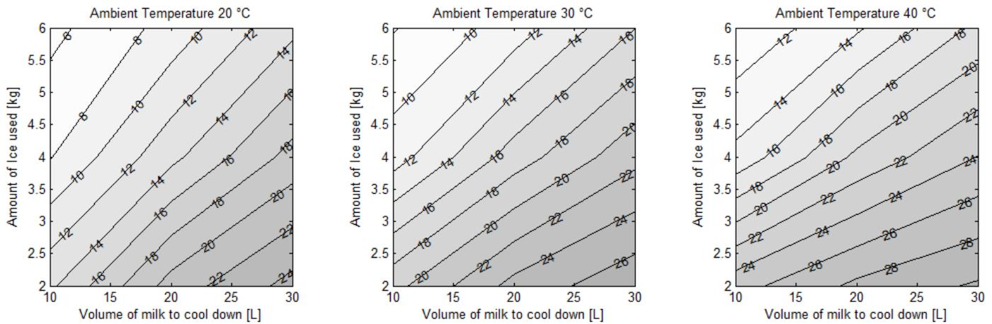
Expected milk temperature 3 hours after milking(36°C). Dependence on milk/ice ratio and ambient temperature.
