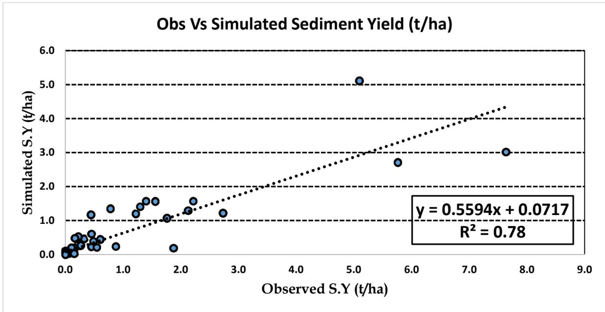
Figure 7.5: Observed and Simulated sediment yield comparison from 2009 to 2011
