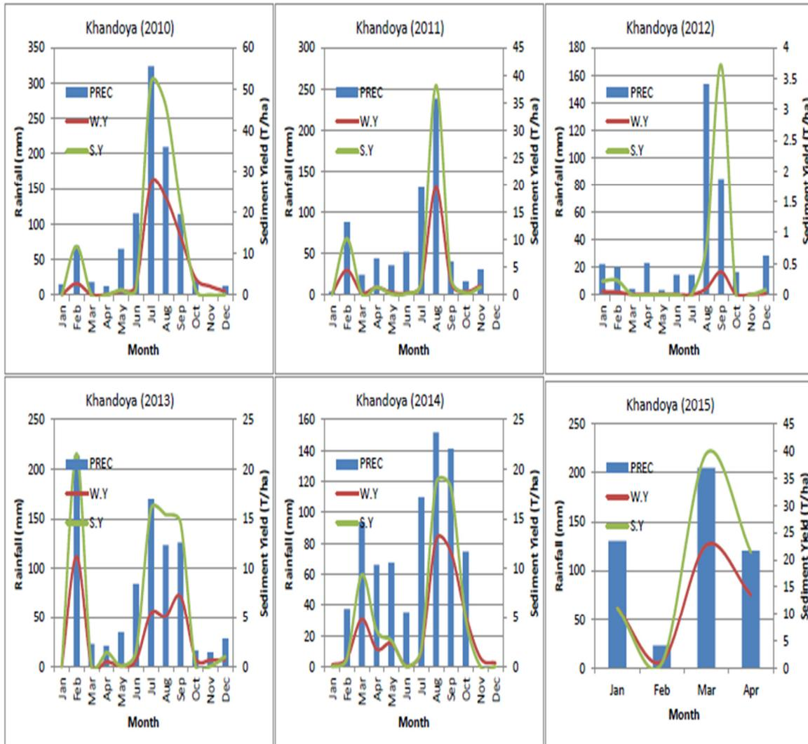
Soil Erosion simulated using SWAT model Khandoya site
