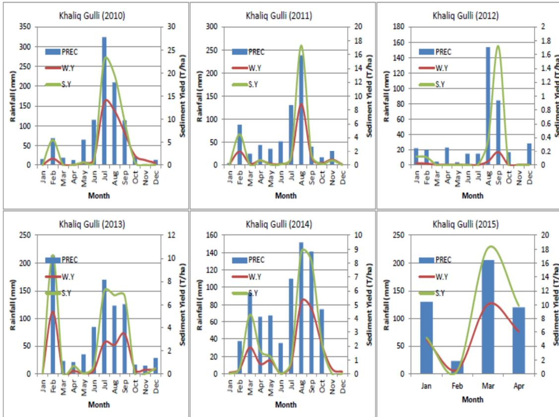
Soil Erosion simulated using SWAT model Khaliq Gully Dhok Mohri site
