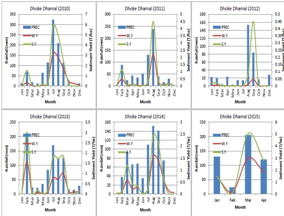
Soil Erosion simulated using SWAT model Dhok Dhamal Fathe Jhang site
