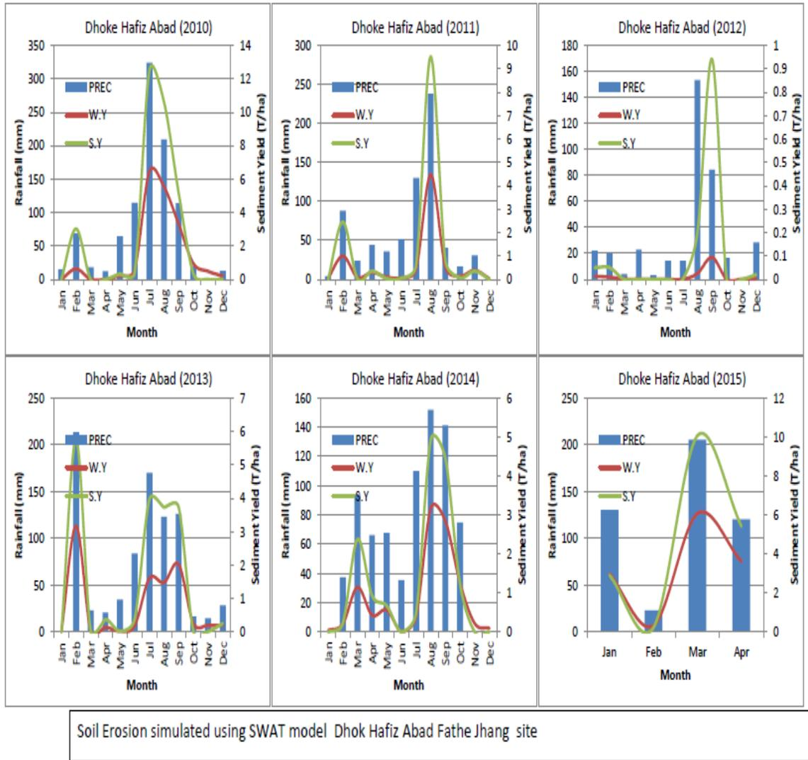
Soil Erosion simulated using SWAT model Dhok Hafiz Abad Fathe Jhang site
