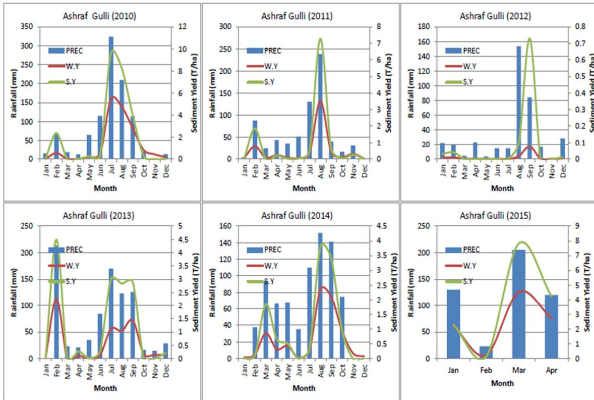
Soil Erosion simulated using SWAT model Ashraf Gully Dhok Mohri site
