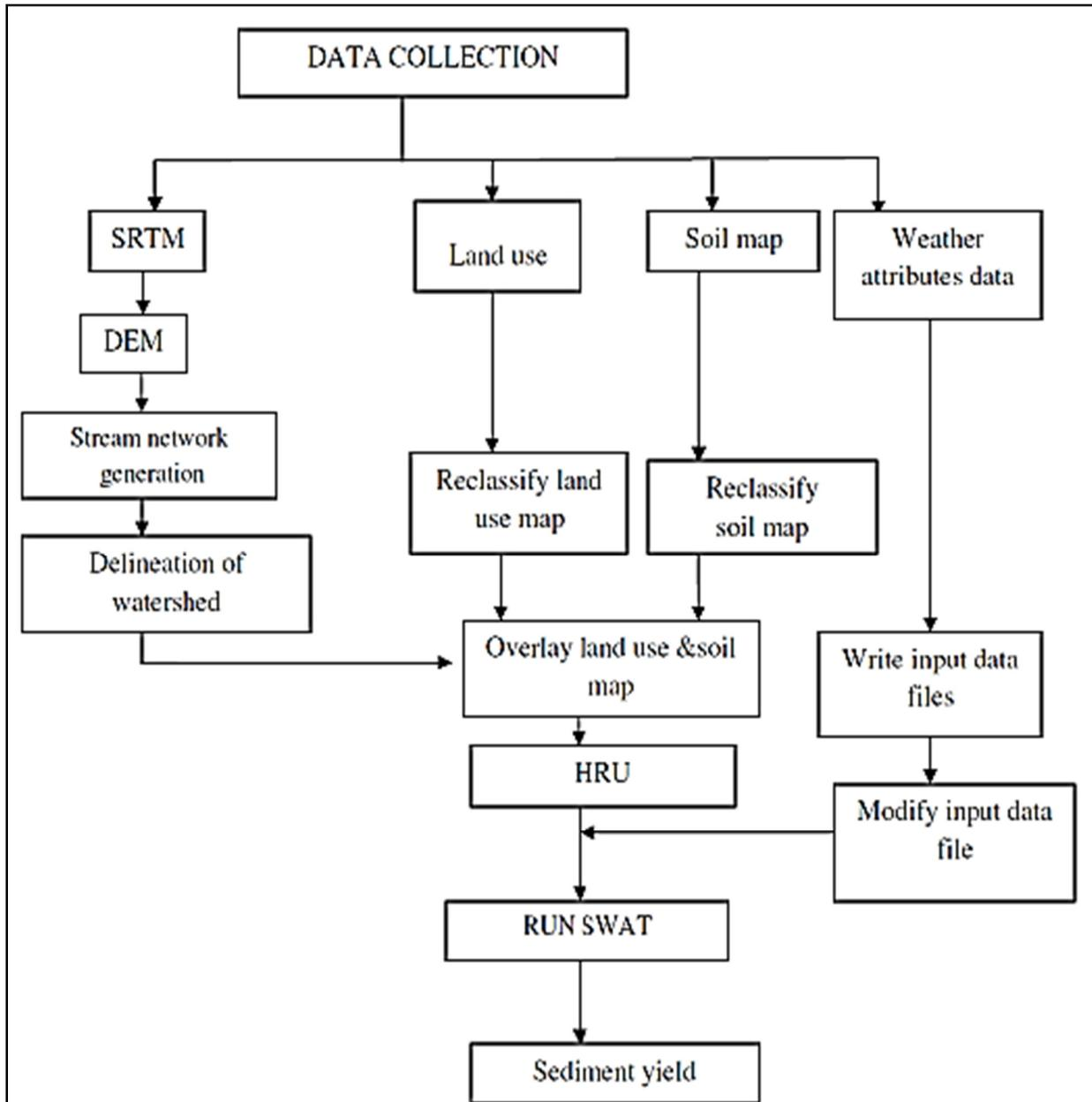
Figure 5-1: General algorithm used for sediment yield simulation in ArcSWAT
