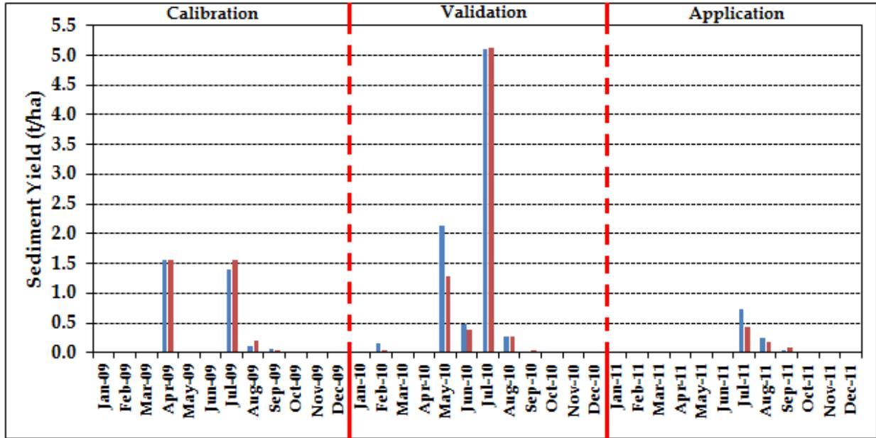
Figure 7.1: Model Calibration, validation and application for catchment 25
