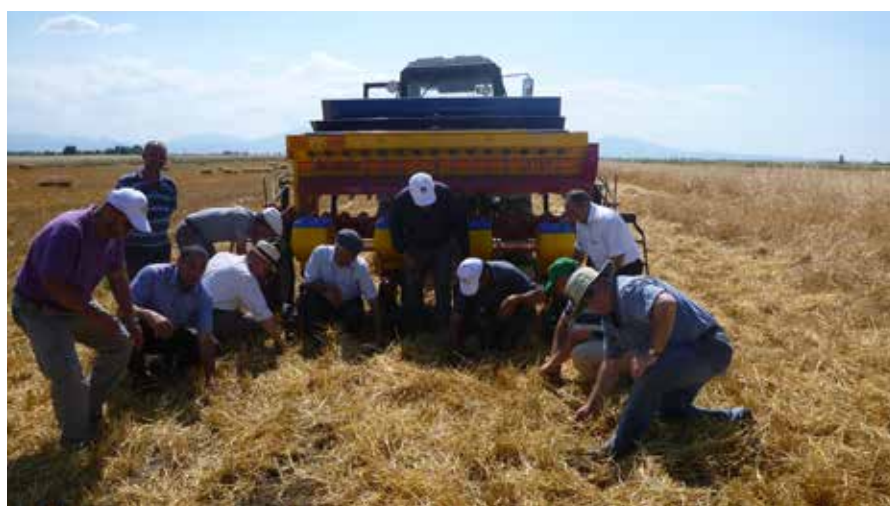
Demonstration of ZT seeding of mung bean in a cereal field in Azerbaijan. Farmers and NARS look for seed placement with ICARDA scientists after sowing with a zero-tillage seeder.
