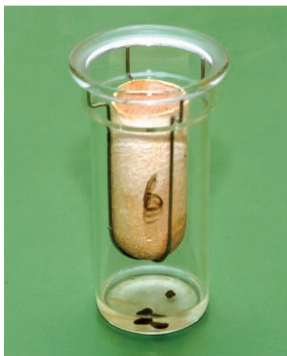
Figure 14. Soxhlet extraction beaker unit with thimble and boiling stones inside
