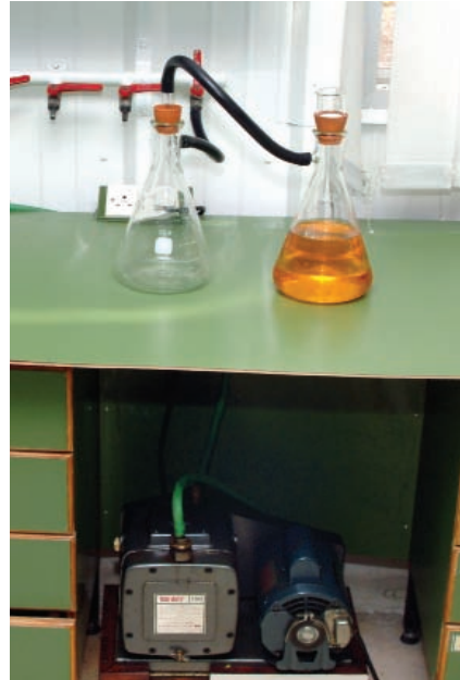
Figure 16. Vacuum filtering system with trap in line
