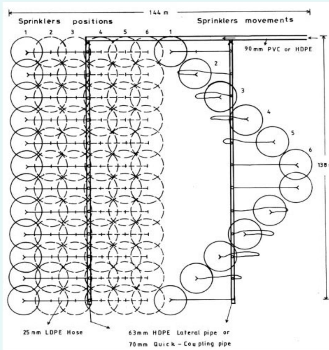
**Typical layout of hose move sprinkler irrigation system (Source: FAO, 2000)**
