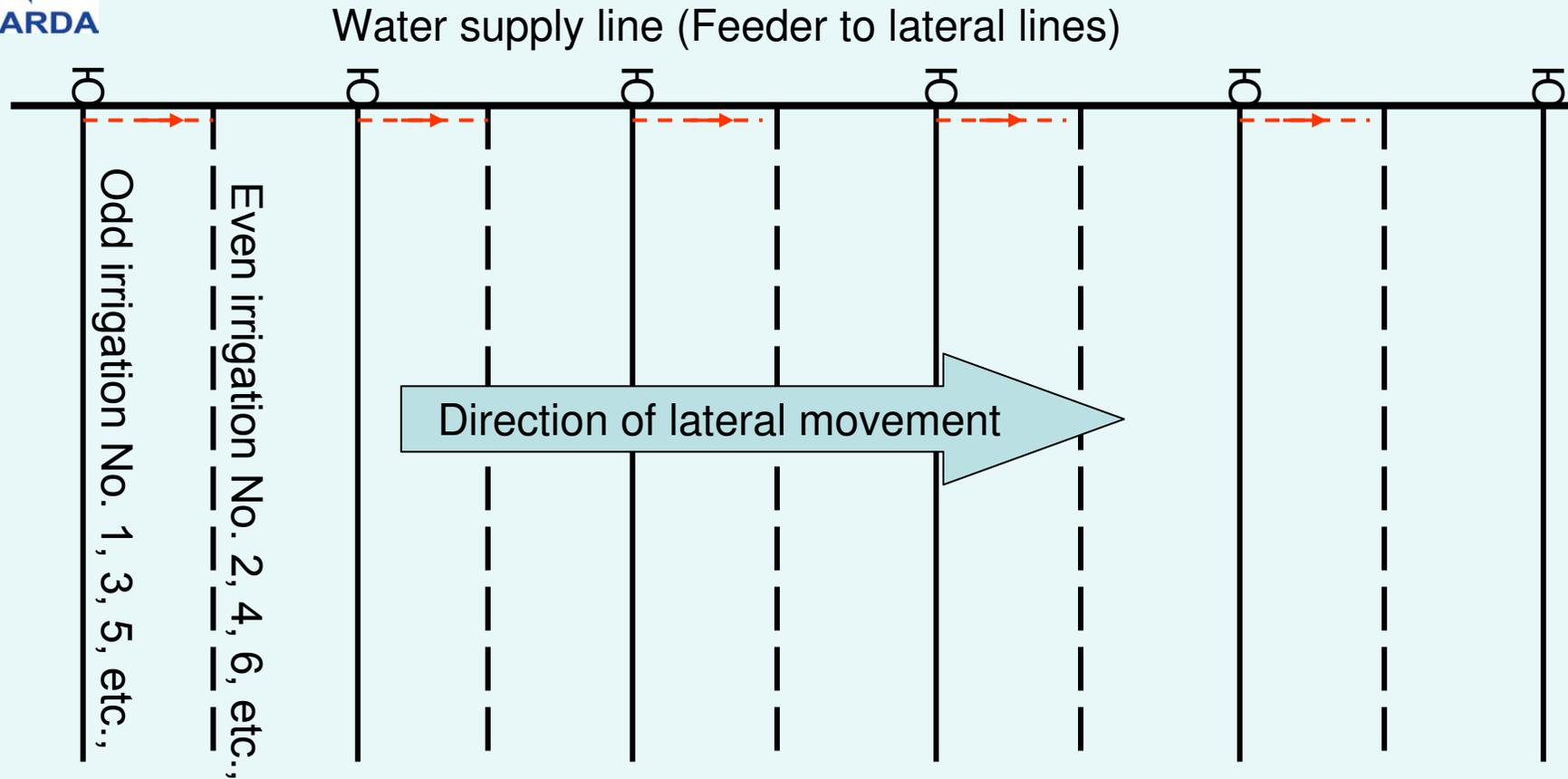
Alternate Setting for Portable Sprinkler Irrigation Lateral lines
